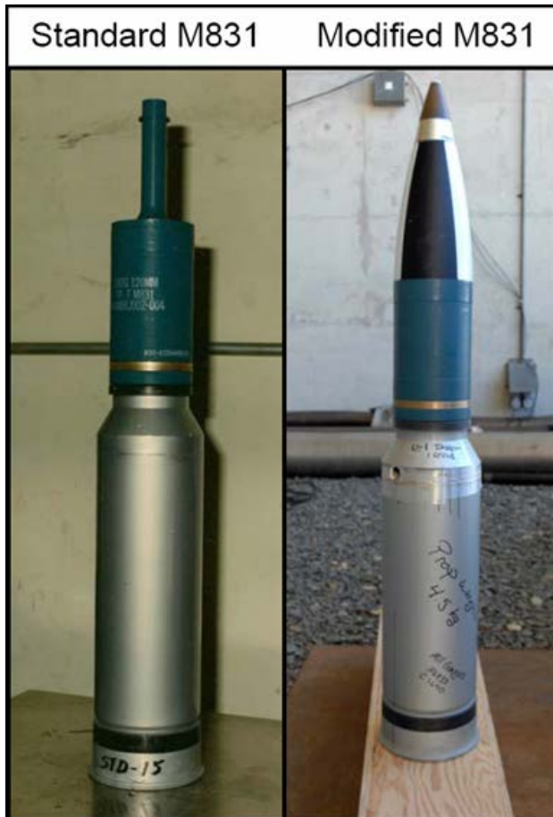
Figure 3. M831 and modified M831 telemetry-enabled high-g carrier with cartridge cases.
