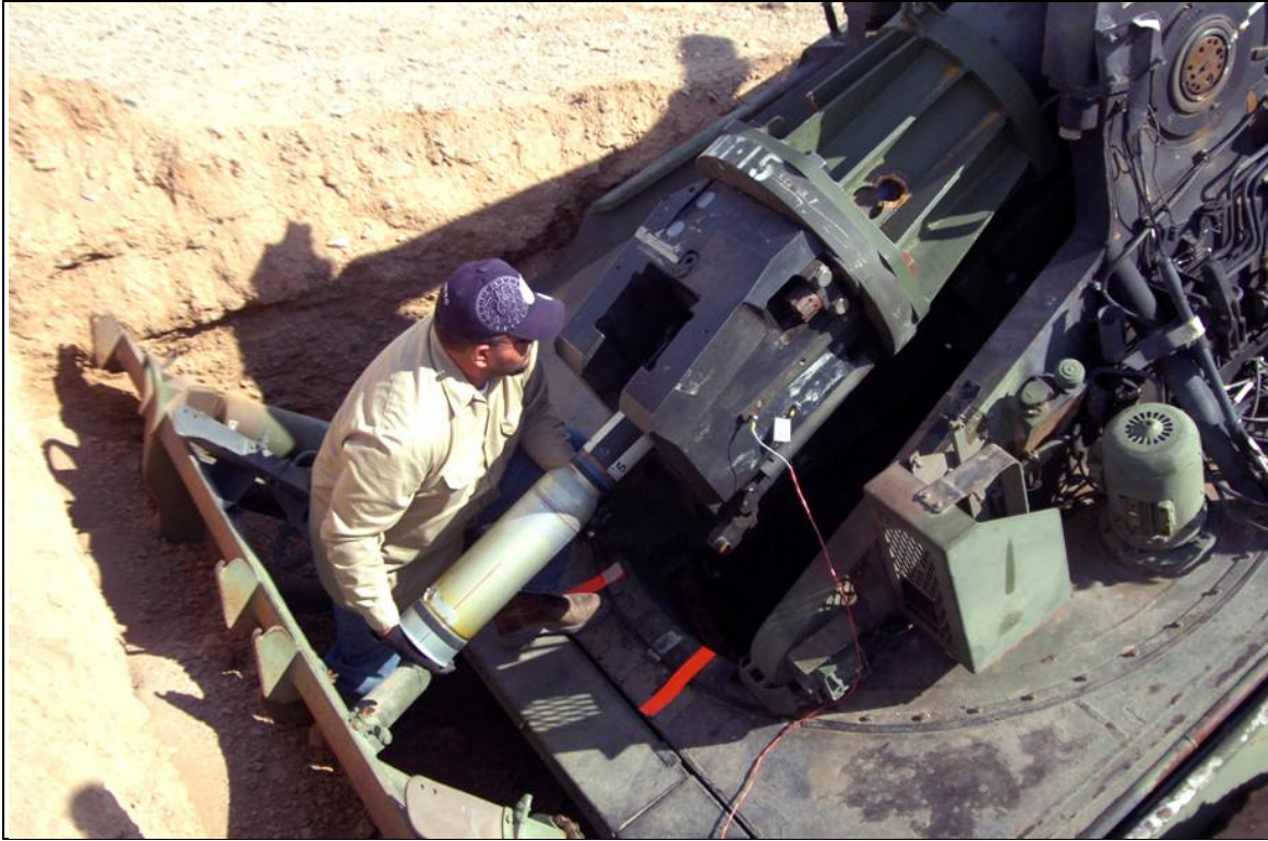
Figure 18. Loading the modified M831 high-G telemetry carrier.
