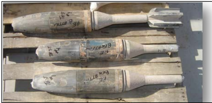
Figure 24. Recovered high-g carrier projectiles.
