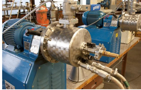
Figure 2. Demonstration of the process scale up going from gram quantity milling (left) to hundreds of grams (right).
