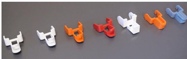
Figure 4. Different generations of rapidly prototyped linkages.
