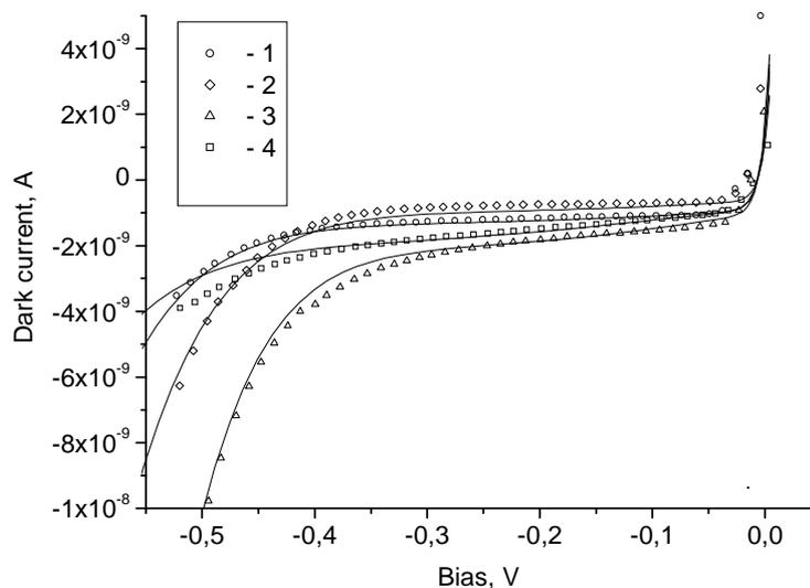
Fig. 6. Experimental (1, 2, 3, 4) and calculated (solid lines) dark current I-V-characteristics of several LPE grown  $\text{Hg}_{1-x}\text{Cd}_x\text{Te}$  ( $x \approx 0.215$ ,  $\lambda_{co} \approx 10.3 \mu\text{m}$ ) photodiodes from different parts of the array.  $T = 77\text{K}$ .
