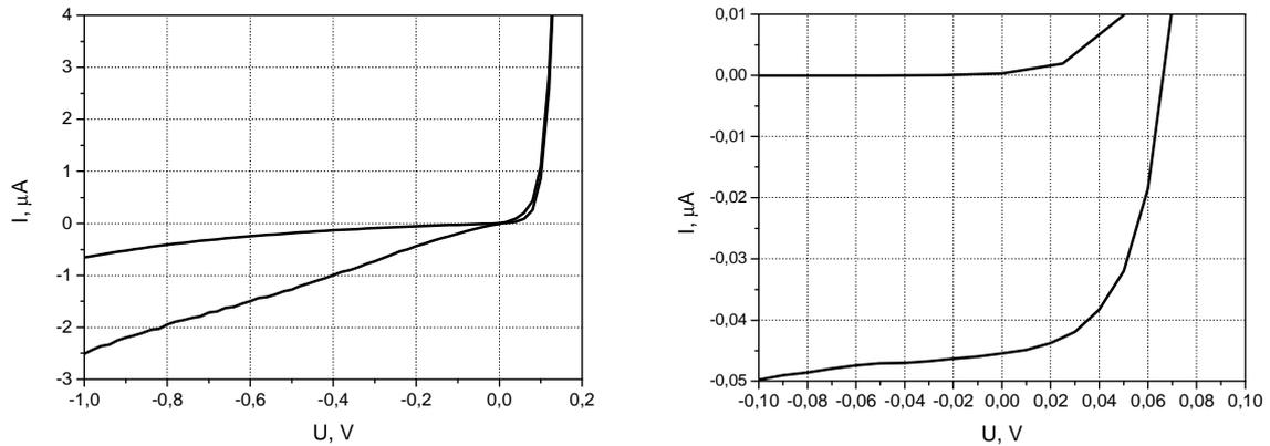
Fig. 7. Experimental dark (1) and background illuminated (2) I-V-characteristic of diode from matrix 128x128, based on  $\text{Cd}_x\text{Hg}_{1-x}\text{Te}$  ( $x \approx 0,3$ ) at  $T=80$  K. Left picture corresponds to LPE grown structures and right image — to MBE manufactured diodes.
