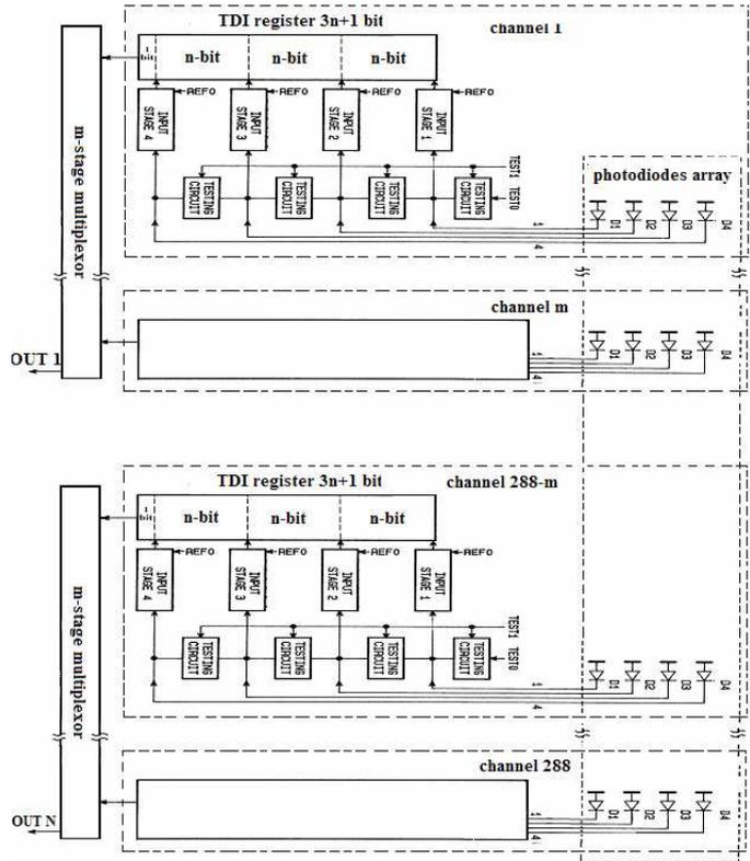
Fig.3. Block-diagram of 4x288 ROIC.
