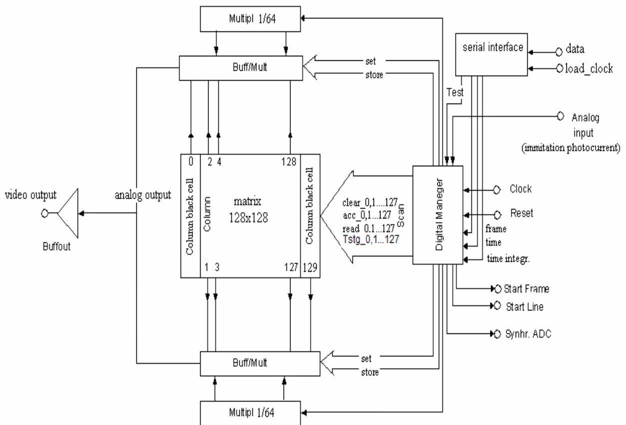
Block circuit readout 128x128.
