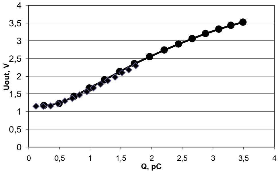
Fig. 3. Transfer characteristic of 4x288 multiplexer.
