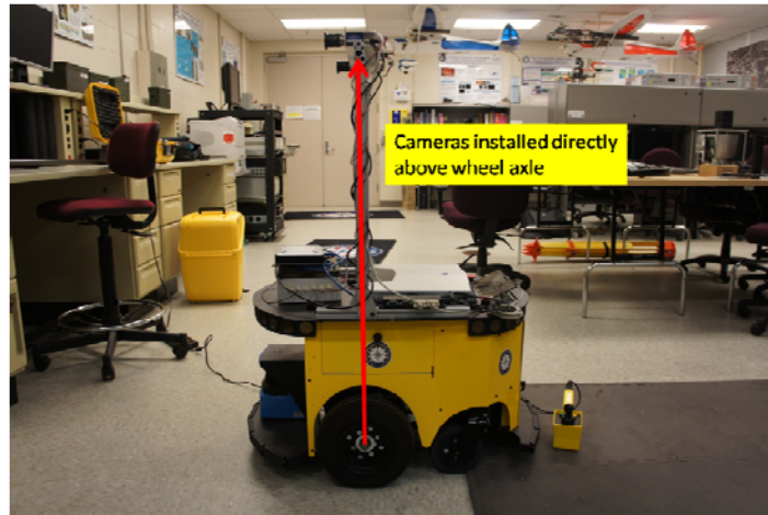
Figure 25: Cameras installed directly above the wheel axle.
