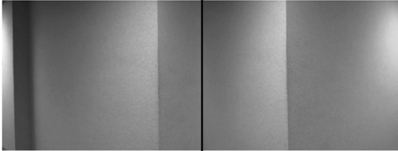
Figure 38: SIFT did not identify any features against a plain wall.
