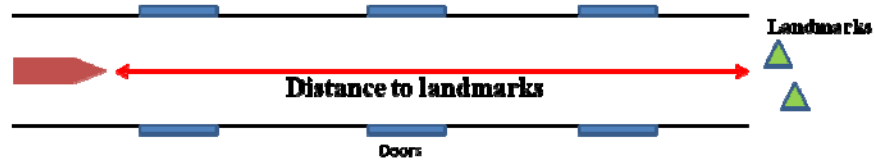
Figure 19: Illustrating the distance to landmarks observed by the robot if it faces straight down the corridor.
