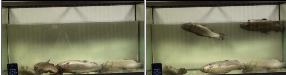
Figure 6. Final Tests of Implanted Tags B9 and B10. Photos show fish prior to and after activation and flotation of fish at day 14.
