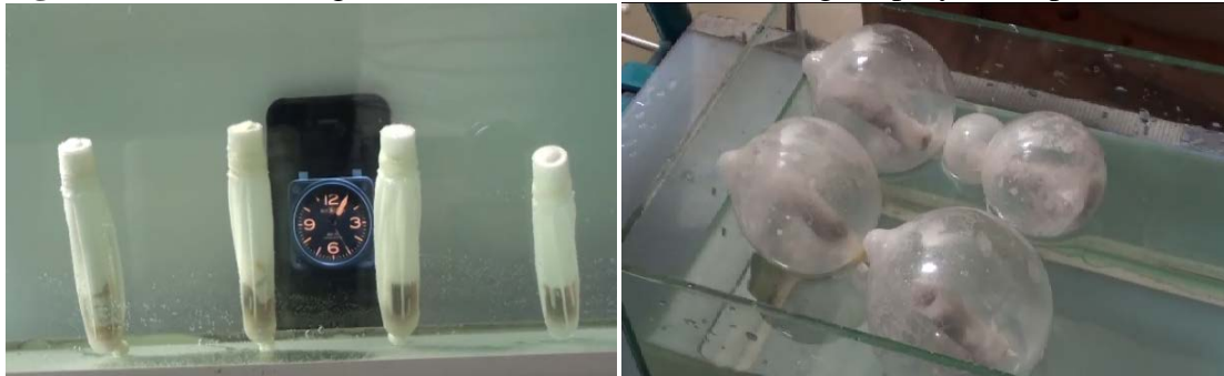
Figure 5. Version 4 Tags Prior to and After Inflation. Tags deployed as specified at 10 days.
