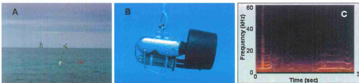
Figure 13: (A) DMON mooring at Horseshoe shoals, Nantucket Sound, site of the first windfarm in the US and one of our DMON passive acoustic monitoring sites. (B) The DMON towfish, a towfish body and fin, with a DMON attached on the underside. (C) Pilot whale whistles and clicks recorded with the DMON towfish.
