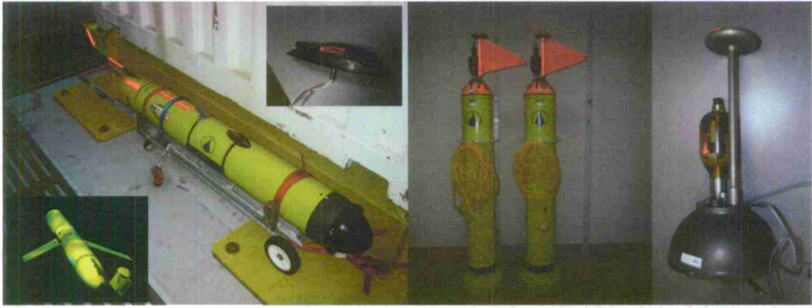
Figure 9: DMON custom integration onto Teledyne Webb glider and profiler
