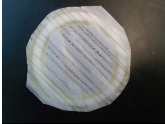
Figure 8. Water Condensation inside the Membrane Assembly
