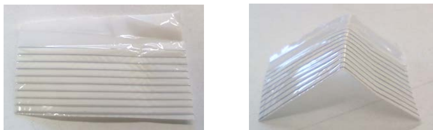
Figure 4. Sample of the Membrane Assembly: Flat (left) and Bent (right)
