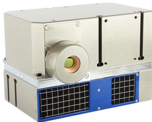
Figure 2: AisaOWL sensor head. The longest dimension of the sensor is 285 mm. Fore-optics is protected against direct heat flow with a removable cover.
