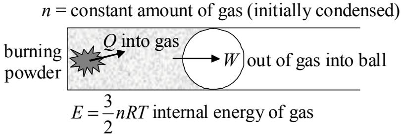
**Figure 3.** Relevant energy transfers between the gunpowder, propelling gas, and musket ball in the model where the number of moles  $n$  of the gas is taken to be constant and its temperature  $T$  increases linearly.
