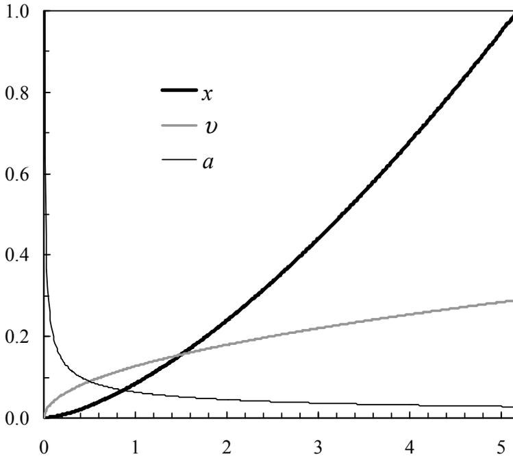
**Figure 2.** Graphs of  $x$  (in m),  $v$  (in km/s), and  $a$  (in m/ms<sup>2</sup>) versus  $t$  ranging from 0 to 5.2 ms if  $k = 5.4 \text{ km}^2 / \text{s}^3$  for the initial conditions  $x_0 = 0$  and  $v_0 = 0$ .
