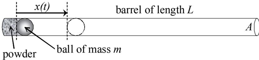
**Figure 1.** Ball in the Barrel of a Musket.
