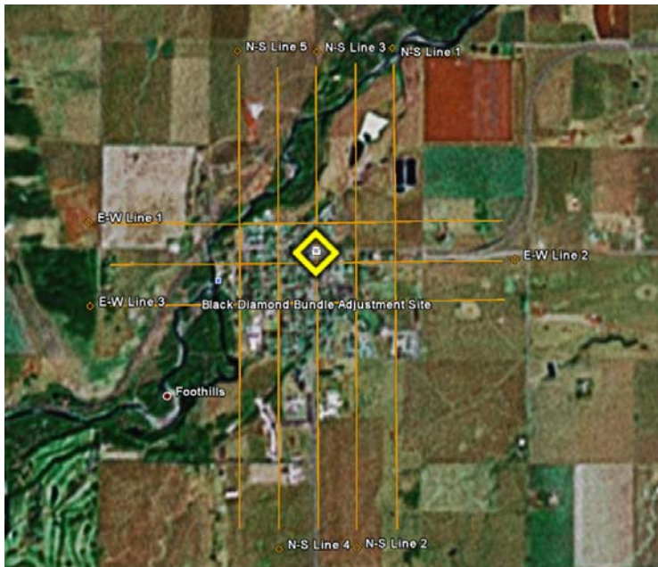
Figure 15: MASI's first test flight plan on Google Earth data
