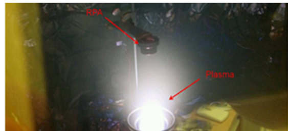
Figure 8 – RPA in plasma in IAD tool
