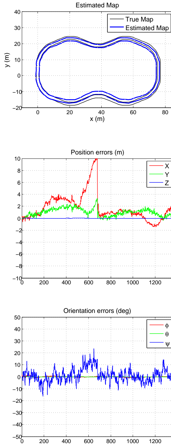
Figure 6.5: Simulation results for map 3: estimated and true map (top), position error (center), and orientation error (bottom).
