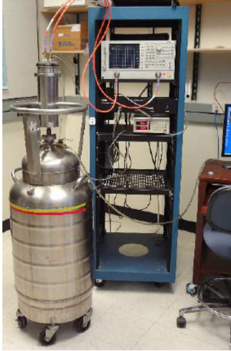
Figure 7: A photograph of the measurement setup, showing the cryostat on top of a liquid helium filled dewar. To the right of the dewar are the VNA, flow control unit, and temperature controller.
