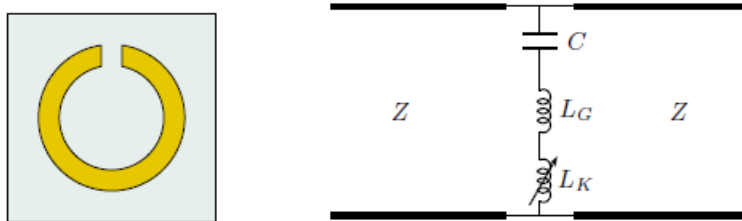
Figure 1: A schematic SSRR (left) and an equivalent circuit (right). C is the gap and surface capacitance, L_G C is the magnetic (geometrical) inductance of the ring and L_K the temperature dependent kinetic inductance of the superconductor.
