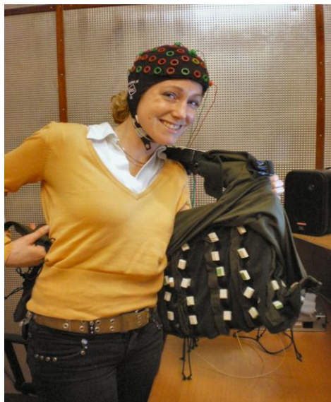
Figure 3: Participant showing the tactile vest and EEG cap used in the experiment.
