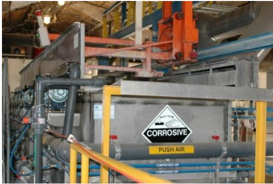
The Base Hydrolysis system utilizes sodium hydroxide to dissolve aluminum containment bodies exposing the CAD or PAD's energetics
