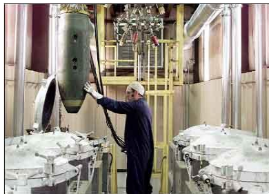
APE 1401M1 Autoclave Meltout (top view); worker directing bomb body into pressure vessel (bottom view)
