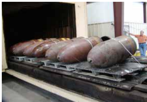
Munitions entering the Hot Gas Decontamination Chamber for removal of residual energetic material
