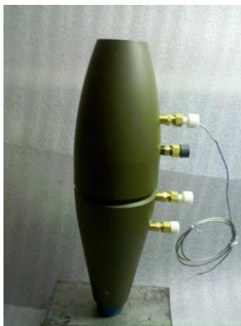
120mm mortar round instrumented with the Ultrasound Melt Cast Inspection System
