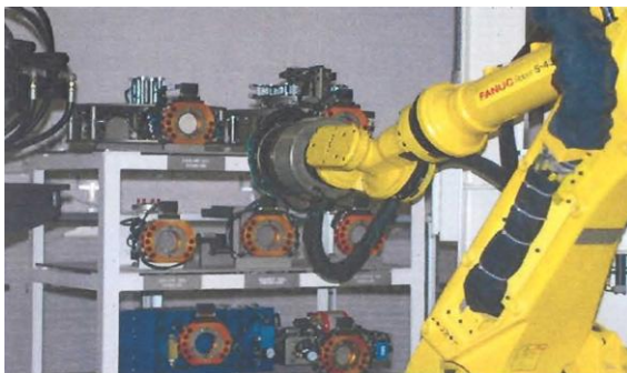
Automated work-cell downloading M42 and M46 submunitions from 155mm DPICM rounds
