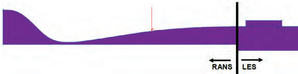
Figure 5. NCPA wind-tunnel nozzle & L/D=6 cavity mounted on the tunnel ceiling
