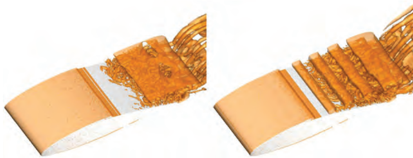
Figure 9. Hybrid RANS/LES simulations for Re=322,000 . Instantaneous iso-surfaces of vortex identification criterion, Q=1 . Uncontrolled flow (left) and controlled flow (right).
