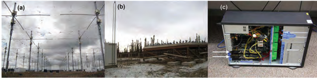
Figure 1. (a) The HAARP ionosphere research instrument (IRI) is collocated with (b) the Modular UHF Ionosphere Radar (MUIR). A workstation at ARSC (b) equipped with two NVIDIA GTX 480 GPU accelerators (indicated with arrows) processed high resolution coded-long pulse data from MUIR.
