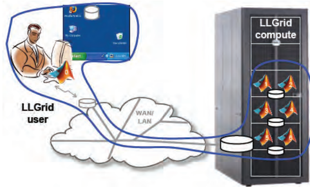
Figure 1. LLGrid file-based parallel computing system. All components of LLGrid are presented to the user via file system abstractions.
