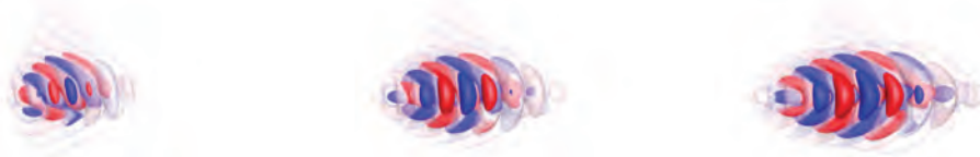
Figure 5. Downstream evolution of wave packet resulting from low-amplitude forcing of oblique mode with \beta=10 . Shown are iso-surfaces of the streamwise disturbance velocity |u'|=10^{-8} and 10^{-9} at t=5.76s (left), 7.68s (center), and 9.6s (right).
