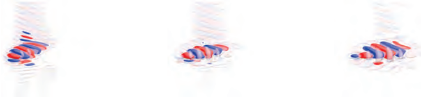
Figure 6. Downstream evolution of wave packet resulting from low-amplitude forcing of oblique mode with \beta=20 . Shown are iso-surfaces of the streamwise disturbance velocity |u'|=2*10^{-9} and 5*10^{-10} at t=5.76s (left), 7.68s (center), and 9.6s (right).
