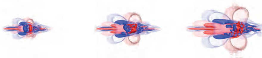
Figure 11. Downstream evolution of wave packet resulting from high-amplitude forcing of oblique modes with \beta=0-40 . Shown are iso-surfaces of the streamwise disturbance velocity |u'|=5 \cdot 10^{-2} and 5 \cdot 10^{-3} at t=5.76s (left), 7.68s (center), and 9.6s (right).
