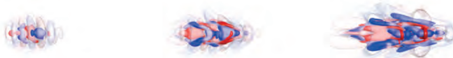
Figure 8. Downstream evolution of wave packet resulting from high-amplitude forcing of oblique mode with \beta=2 . Shown are iso-surfaces of the streamwise disturbance velocity |u'|=5*10^{-2} and 5*10^{-3} at t=5.76s (left), 7.68s (center), and 9.6s (right).
