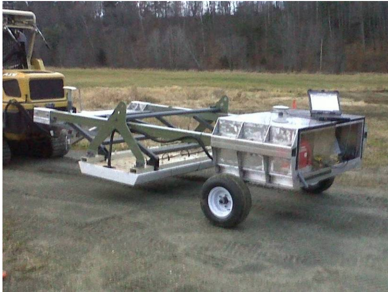
Figure 6. The ARA/NED UXO Trailer Towed by the ARTS.
