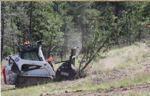
Figure 37. Team D4C Bobcat Midsize Vegetation Removal and Mowing
