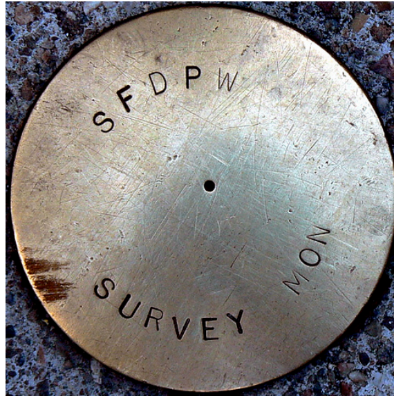
Figure A-11: Example Picture of a Surveying Monument (From Google Image Search.)
