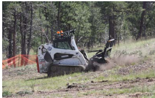
Figure 37. Team D4C Bobcat Midsize Vegetation Removal and Mowing
