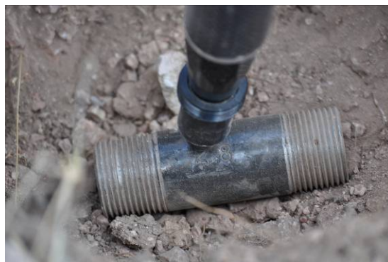
Figure A-10: Example of Sub Surface UXO Placement & GPS Measurement.
