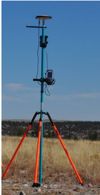
Figure A-8: Physical Setup for Base Station.
