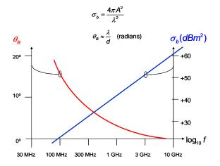
Figure 2: Forward scatter RCS  $\sigma_b$  and angular width  $\theta_F$  of scatter for a typical small aircraft target  $(A = 10\text{m}^2, d = 10\text{m})$ .
