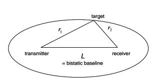
Figure 1: Bistatic geometry [35].
