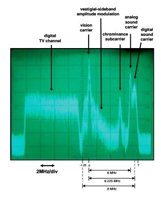
Figure 6: Spectrum of typical PAL analogue TV signal (right of centre) and digital TV signal (left of centre). Horizontal scale 501–521 MHz; vertical scale 10 dB/division.
