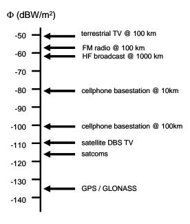
Figure 11: A 'league table' of some passive bistatic radar illumination sources, arranged in order of power density at the target. These power densities have been calculated on the basis of a single channel, full signal bandwidth, no processing gain and free space propagation (except for the HF broadcast signal, for which the propagation, and hence the power density, will depend on time of day, season and time of sunspot cycle).
