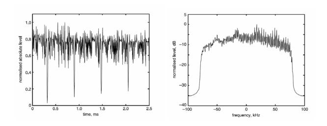
Figure 8: (a) time-domain representation of part of one TDMA-modulated carrier of a GSM signal, showing the 577 µs slots; (b) frequency-domain representation, showing the 200 kHz channel (after Tan et al. [49]).
