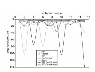
Figure 5: Variation in range resolution as a function of time for seven types of VHF FM radio modulation over a two-second interval (after [\*]).
