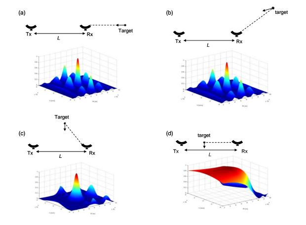
Figure 3: Bistatic ambiguity functions for four different target locations and directions of motion.
