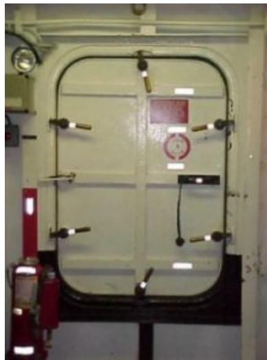
Figure 36. Water-tight Door and Bulkhead From [92]
