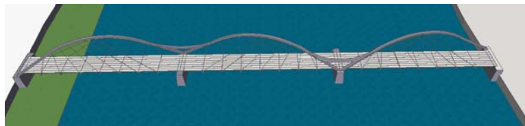
Figure 32: Swooping Arch Sections Installed
