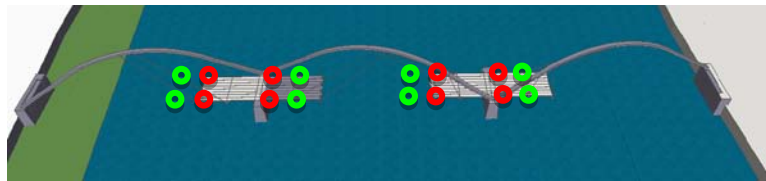
Figure 29: Interior deck sections installed
