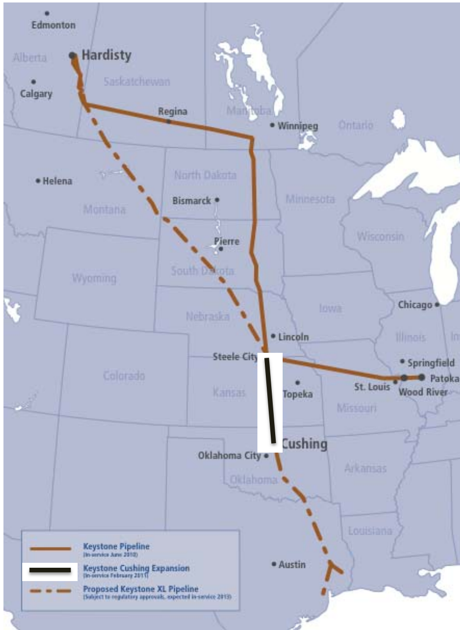
Figure 4. The proposed Keystone-XL Pipeline Route. The Keystone Cushing Expansion Extended the Keystone Pipeline System from Steele City, Kansas to the COH. Adapted from TransCanada. 48
