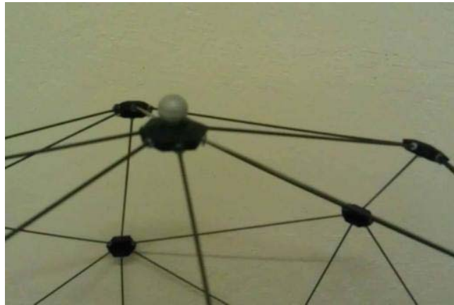
Figure 26. Reflectors on the UAV
