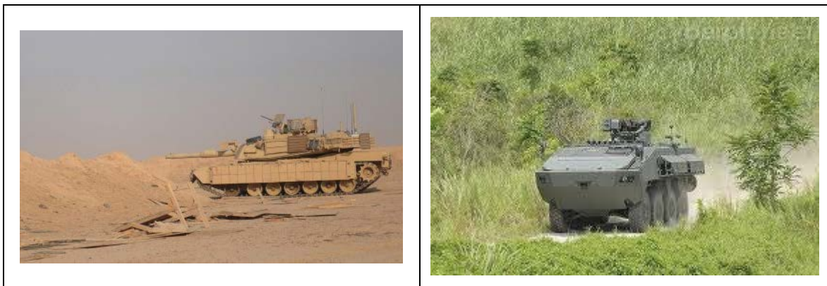
Figure 55. Reduction of Visual Signature: M1A2 Abrams (left) in a Desert Environment (From U.S. Army 2011) vs Terrex Infantry Carrier Vehicle (Right) in a Jungle Environment (From Ministry of Defence, Singapore 2009).
