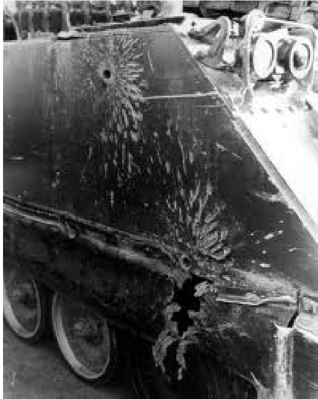
Figure 12. An M113 with Hits from a Viet Cong 57mm Recoilless Rifle (From Starr 1980, 46)
