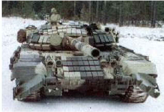
Figure 58. T-72 Tank with Reactive Armor (From Federation of American Scientists 2000)
