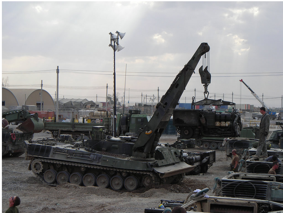
Figure 66. Buffel ARV Lifting a Leopard 2 MBT Engine (From Defense Industry Daily 2012)
