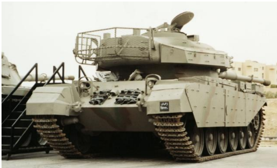
Figure 41. A Jordanian Centurion MBT (Note the Side Skirt) (From IHS Jane's 2012)
