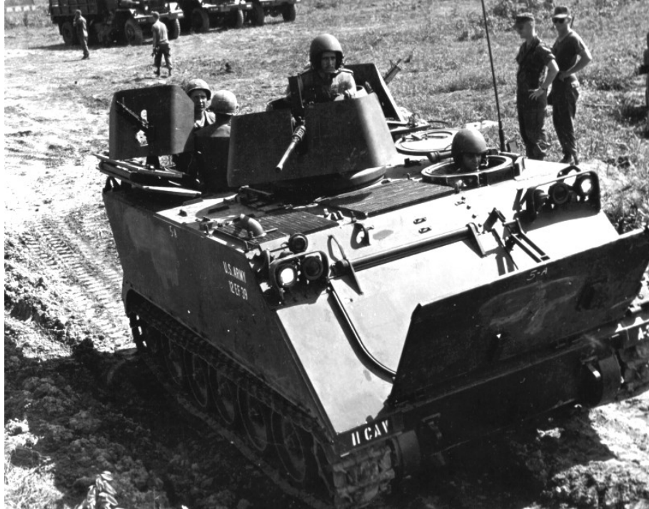
Figure 11. A M113 with a Gun Shield Modification (From Starr 1980, 74)
