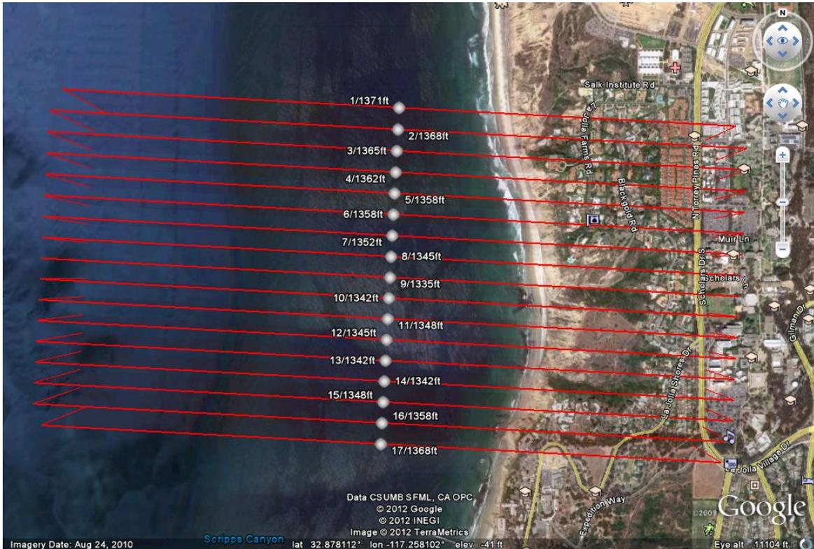
Figure 16. Planned flight lines for the high spatial resolution collection (From Goodrich ISR Systems, 2012)
