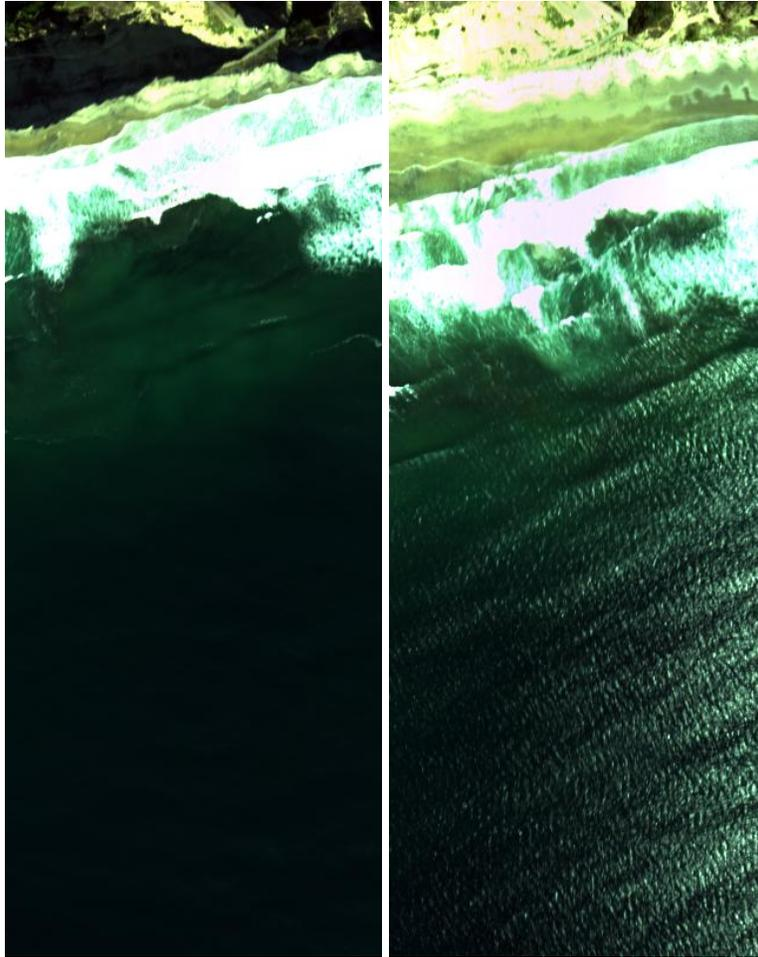
Figure 10. True color composite images (R: 641 nm, G: 551 nm, B: 460 nm) from ProSpectIR-VS3 illustrating the effect solar elevation angle has on glint. Both images were recorded by the same sensor, with the left image being recorded early in the morning and the right image recorded mid-day
