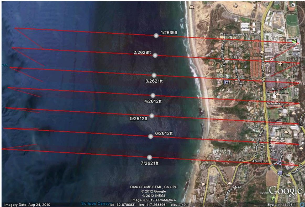
Figure 17. Planned flight lines for the low spatial resolution collection (From Goodrich ISR Systems, 2012)
