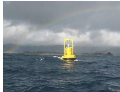
Wave energy generating “PowerBuoy” – Kaneohe Bay
