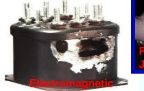
**Relay Vapor Arc Damage**
