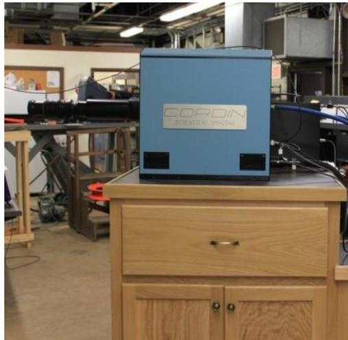
Figure 3. The Cordin Company Model 570 digital color framing camera.
