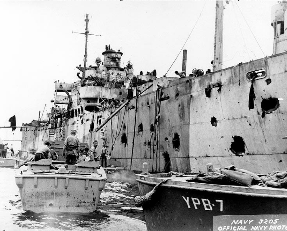
Photo # NH 96174 Damage to USS Mindanao from Mt. Hood explosion
