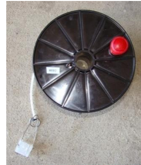
Detachment at Reed Valve Stem (Lost 1 sample out of 10)
