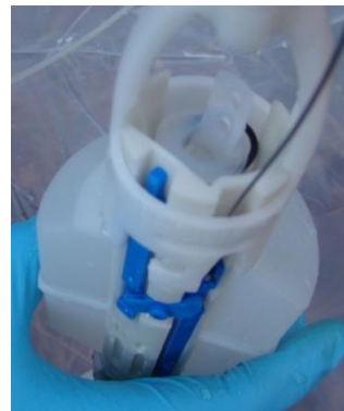
Incomplete Closing of Snap bottle (1 of 28)
