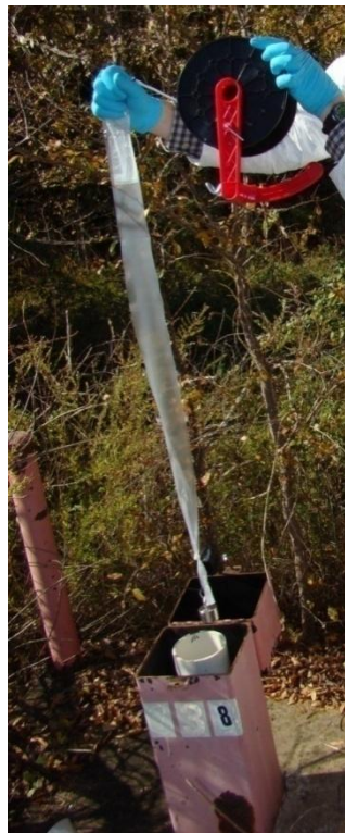
Deployment (Right) and Retrieval (Left) of the HydraSleeve Sampling Technology
