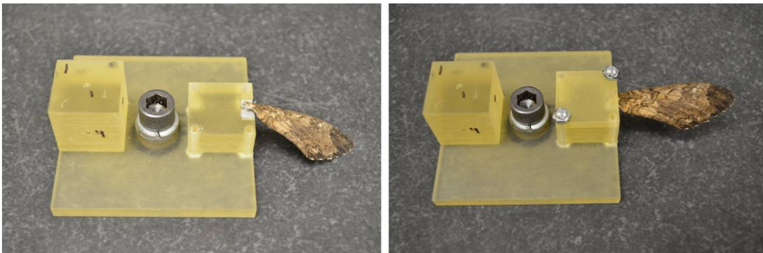
Figure 42: Alignment Jig with Wing Unclamped and Wing Clamped
