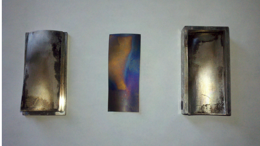
Figure 54: Machined Aluminum Mold with Sample Nitinol Sheet
