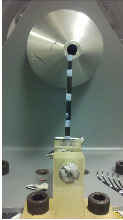
Figure 65: 40 mm x 2.5 mm beam with airhorn excitation
