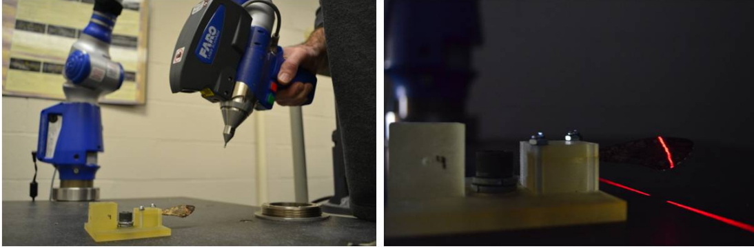
Figure 43: Faro Laser Line Scanner Actively Scanning Wing
