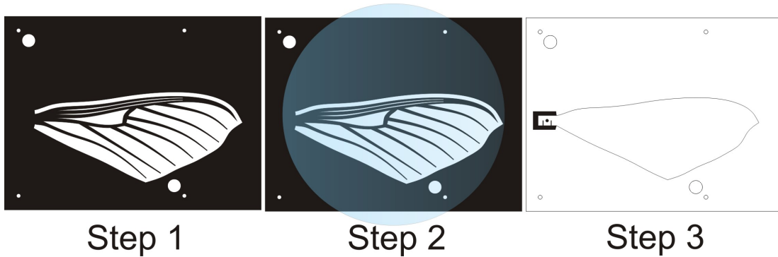
Figure 89: Venation Cutting Pattern and Venation/Membrane Release Pattern
