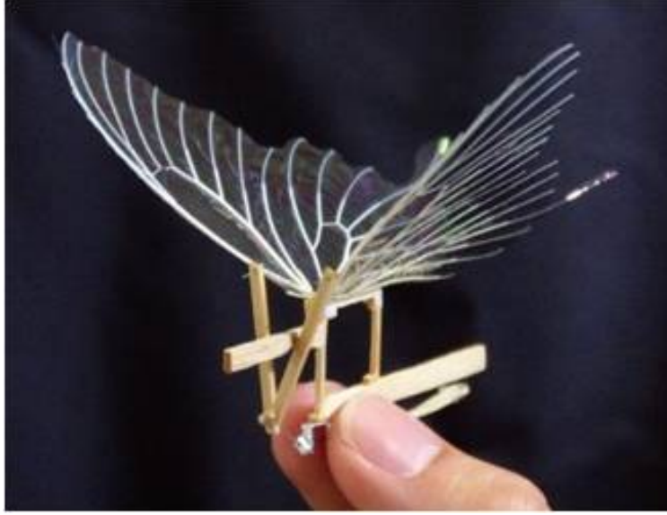
Figure 24: Tailless Ornithopter Mimicking a Swallowtail Butterfly [92]
