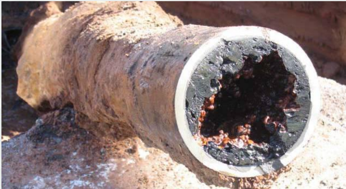
Tuberculation in 6-inch Unlined CI Water Main
