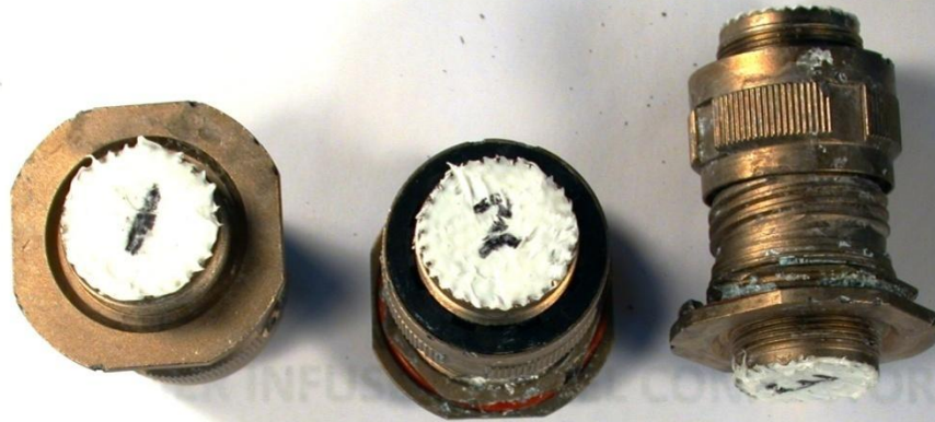
POLYMER INFUSED NICKEL CONNECTOR ASTM B117 452 HRS MATED - 48 HRS UNMATED RINSED AND CLEANED
