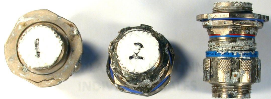
ALUMINPLATE TRI CR CONNECTOR ASTM B117 452 HRS MATED - 48 HRS UNMATED RINSED AND CLEANED
