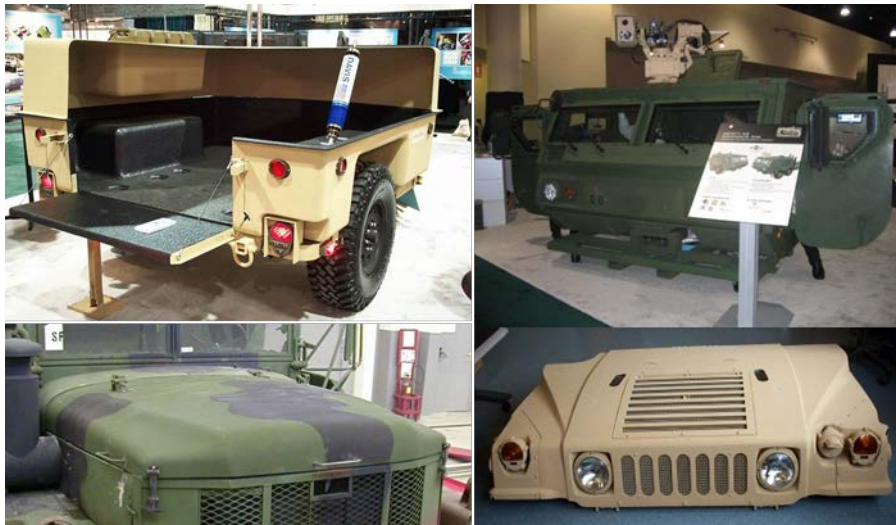
Figure 1 Example Composite Structures fabricated using Liquid Composite Molding processes.
