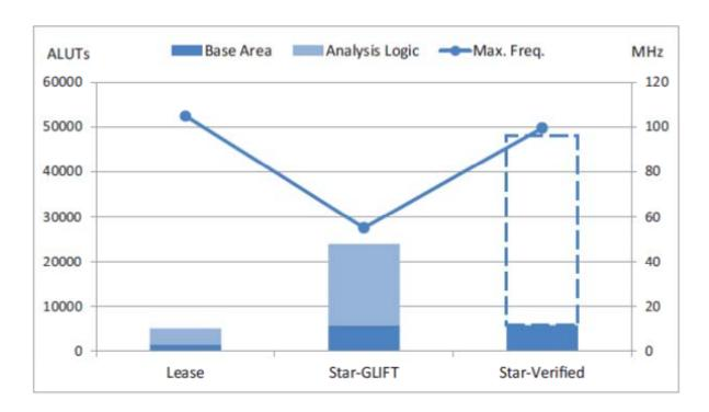
The above graph quantifies the size and performance advantages of the Star-CPU against the Execution Lease CPU and against the Star-CPU with dynamic GLIFT logic (Star-GLIFT). The Star-CPU provides caches, pipelining, and kernel support beyond the Lease CPU in equivalent area and clock-frequency, and provides static security guarantees compared to Star-GLIFT in almost 1/4 the logic, 1/2 the memory, and 2X the clock-frequency.
