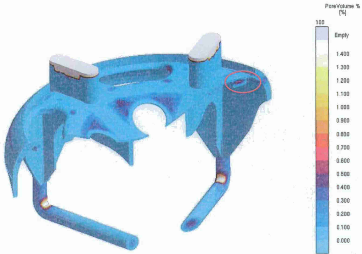
Figure 2 Porosity prediction for mortar baseplate casting simulated using the advanced feeding development model in MAGMAsoft. Worst porosity for section indicated.
