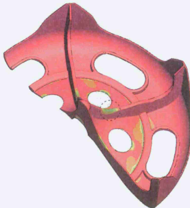
Figure 25 Fatigue life prediction without including effects of porosity gives minimum fatigue life of 12,900 cycles of load case 80 degrees over no spade. Also twenty nodes had lives < 40,000 cycles.
