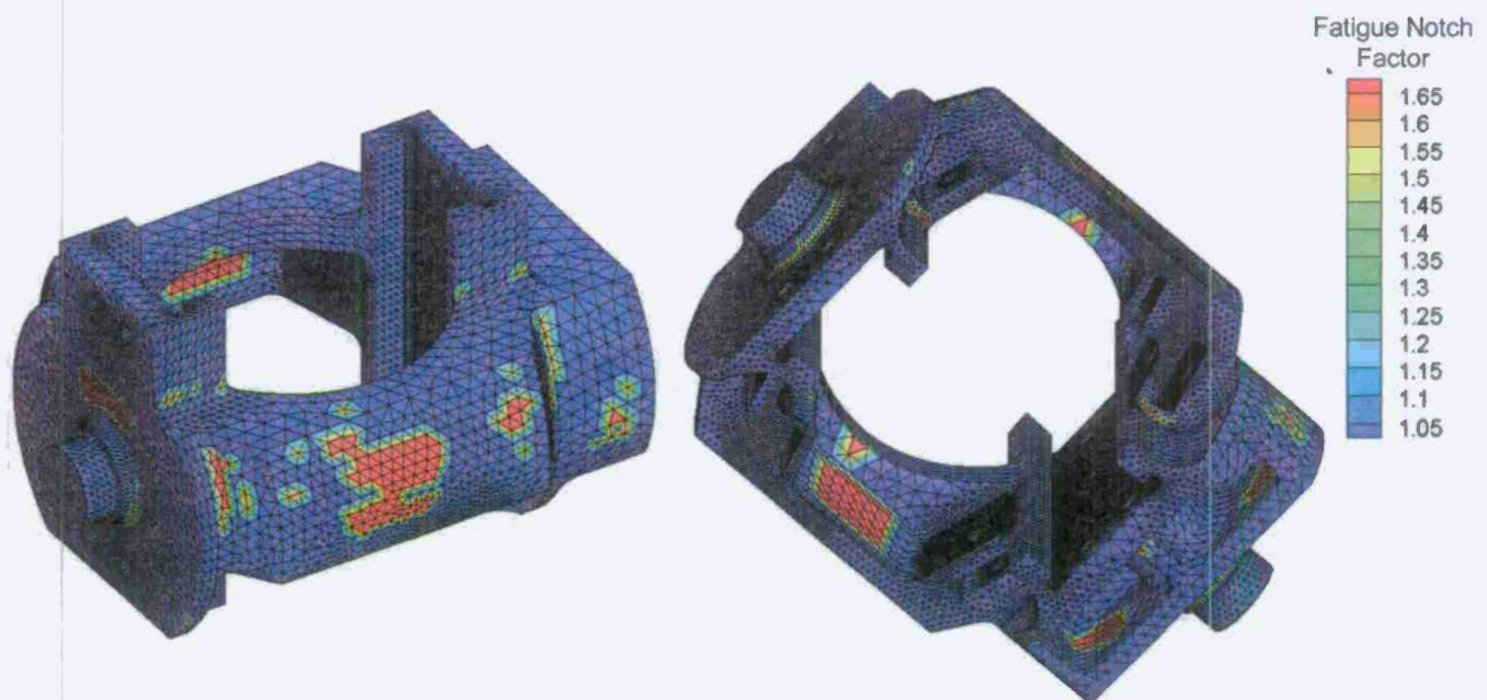
Figure 9 Fatigue notch factor determined from the microporosity results is mapped onto FEA mesh. Microporosity porosity results are used to predict part performance since they appear to be the most sensitive and are worst of the three (most conservative).
