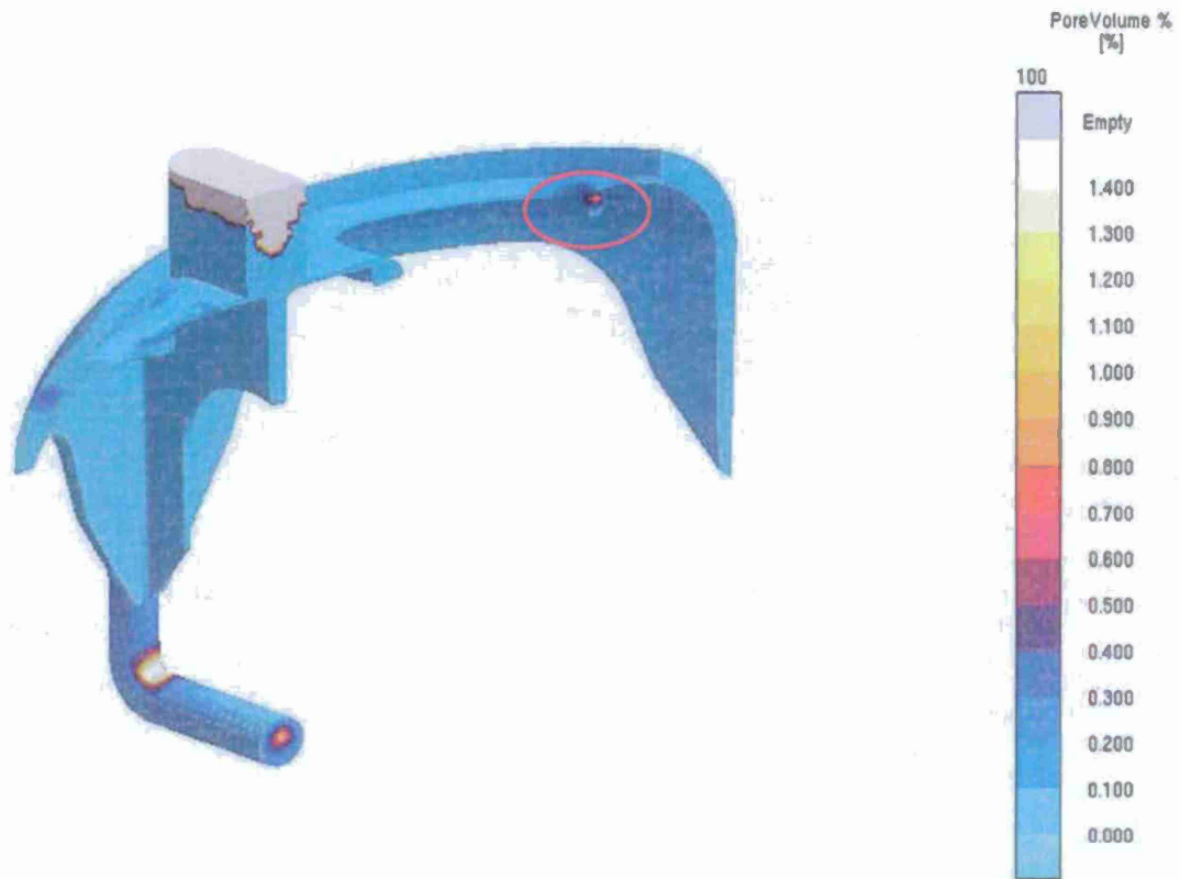
Figure 4 Porosity prediction in mortar baseplate casting simulated using the advanced feeding development model in MAGMAsoft. Worst porosity for section is indicated indicated.
