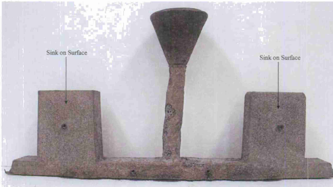
Figure 13 Picture of one of the three (out of four) castings determined to have visible surface sinking. This indicates external shrink. Note the thermocouple locations are seen at the dark round holes.
