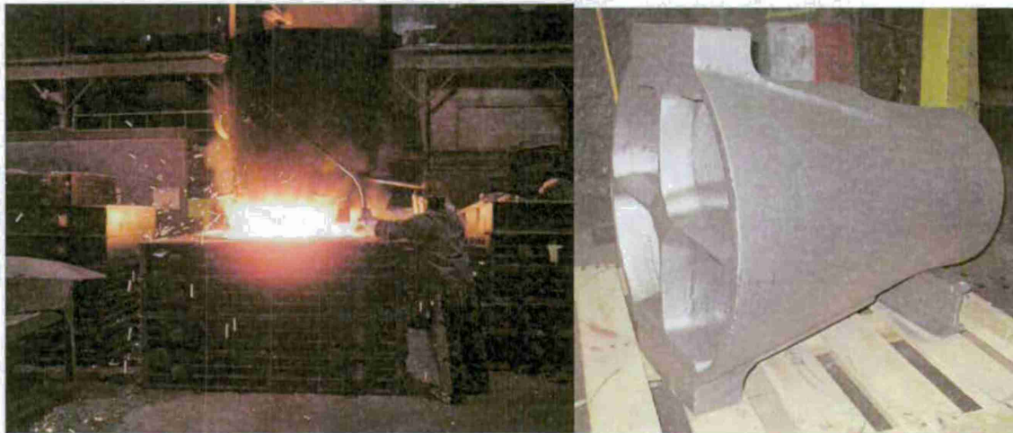
Pouring of prototype breech nozzle and as-cast part.
