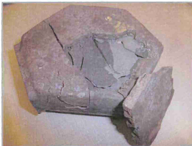
Spokane pour 2 with 8630 and Si-C shows both reaction and cracking of both metal and tile
