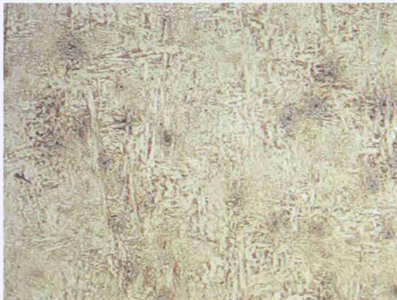
Figure 5: As cast microstructure of 4330steel in low magnification 200X
