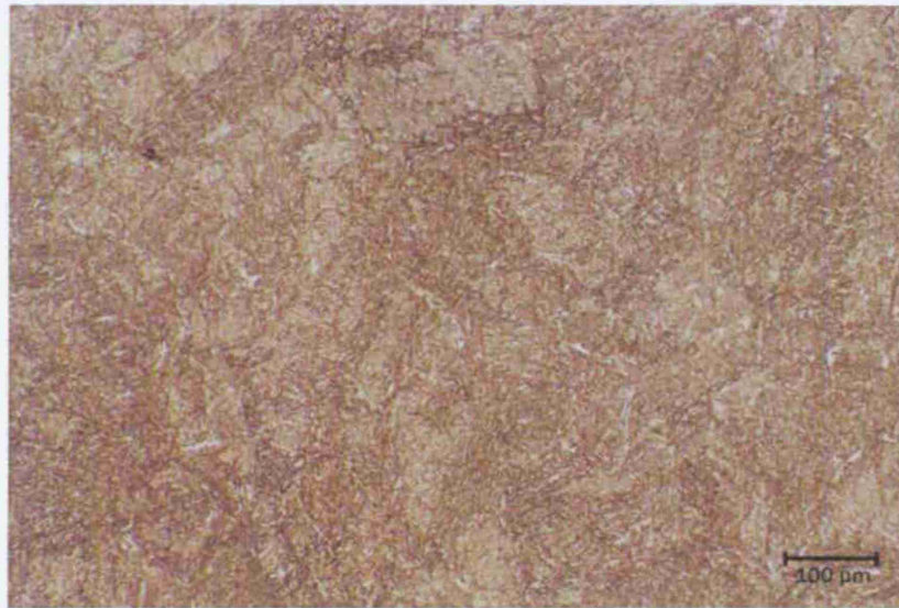
Figure 5 Micrograph of carrier piece showing lath-martensitic structure with no inclusions.
