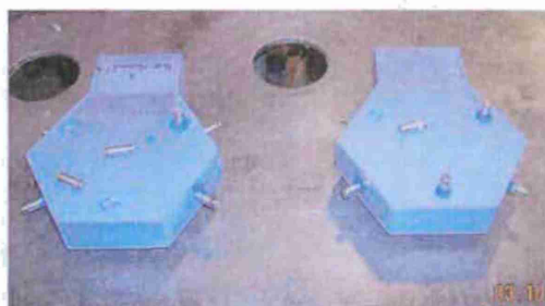
SiC Armor Disc Encapsulated with FOPAT Patterns with Stainless Steel Locating Pins
