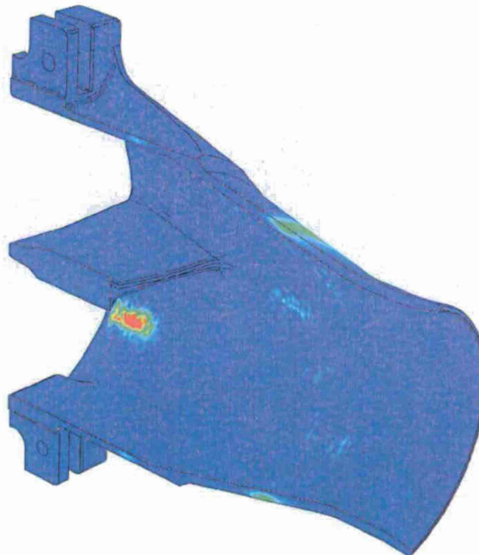
Figure 12 Porosity fraction for re-designed breech nozzle mapped onto ABAQUS finite element mesh with center tube cut away showing higher level of porosity.
