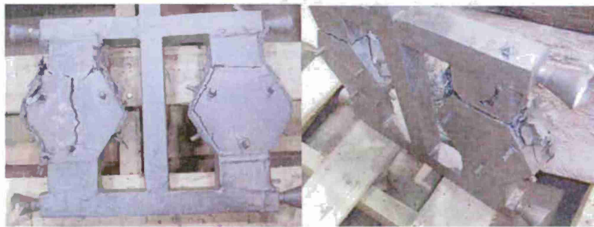
Casting After Pouring Just After Shell Removal Showing the Hot Tearing
