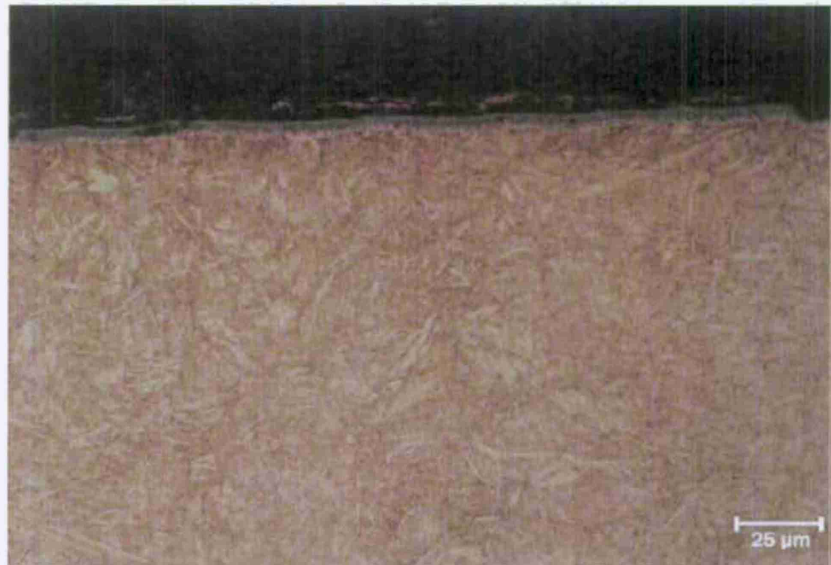
Figure 2 Micrograph of carrier puck showing a microstructure free of primary carbides.
