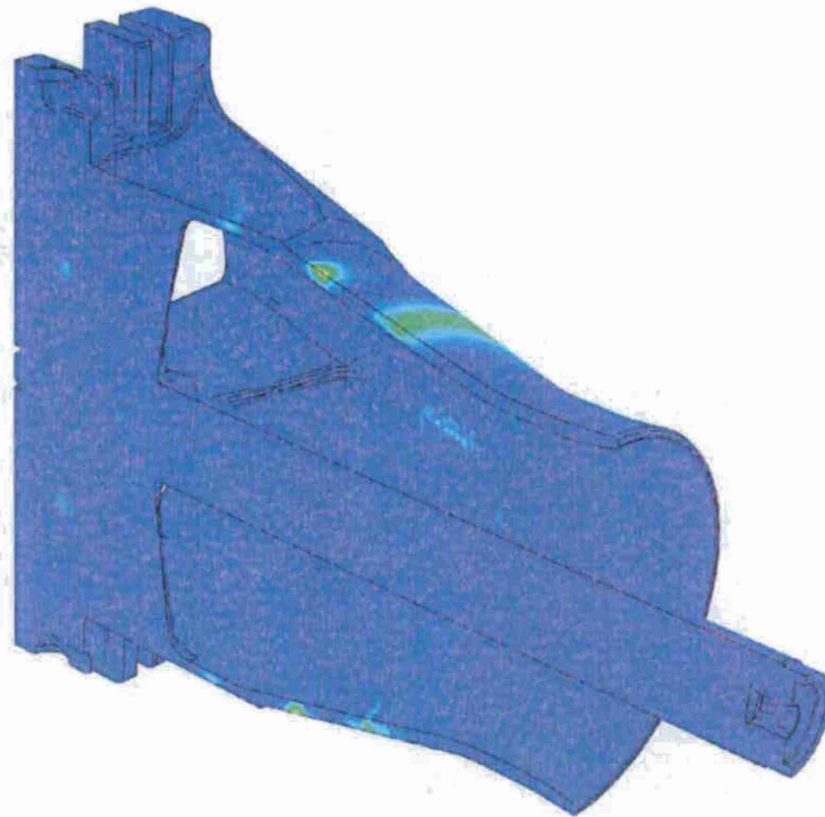
Figure 11 Porosity fraction for re-designed breech nozzle mapped onto ABAQUS finite element mesh.
