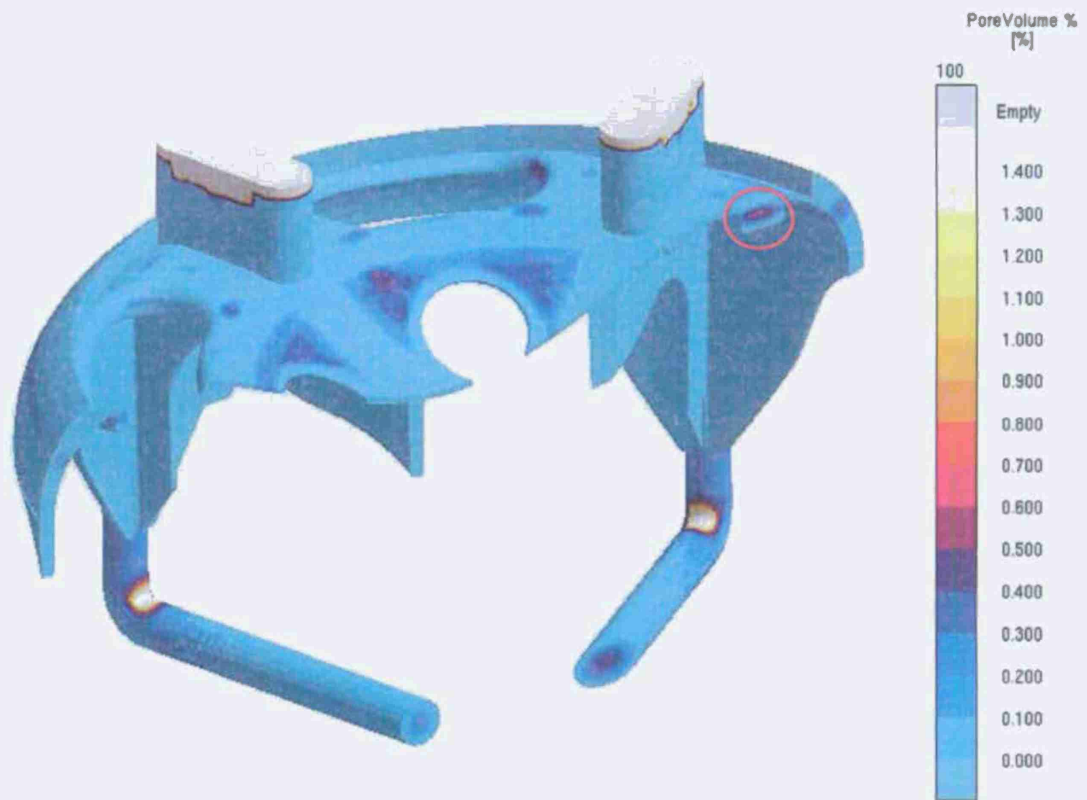
Figure 22 Porosity prediction for mortar baseplate casting simulated using the advanced feeding development model in MAGMAsoft. Worst porosity for section indicated in red circle.
