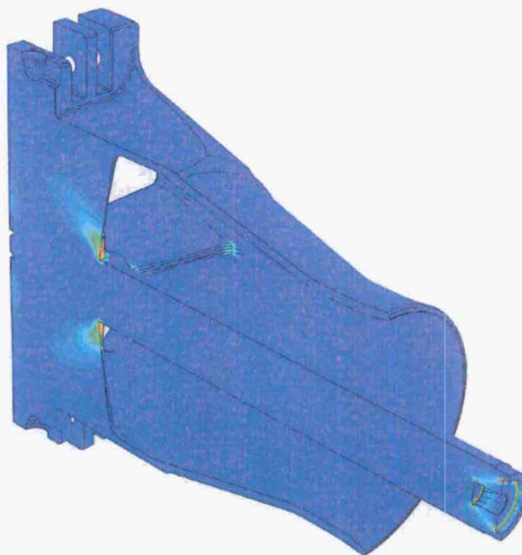
Figure 10 Equivalent plastic strain for re-designed breech nozzle using elastic-plastic analysis.
