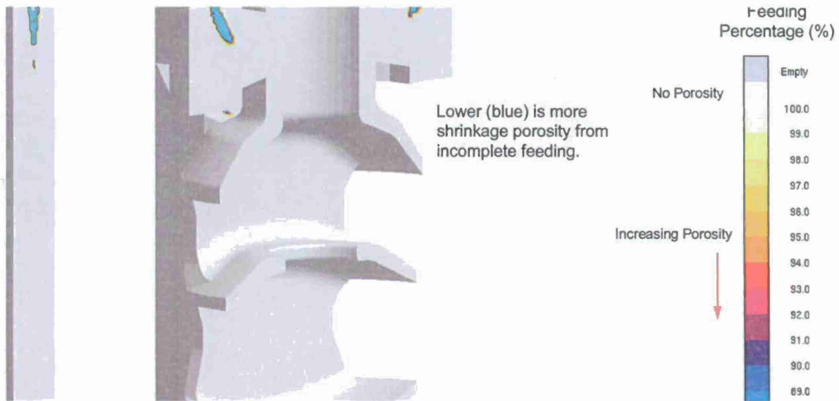
Figure 2 Feeding Porosity predictions in center slices across the casting and risers to show riser pipes. Casting had no shrinkage indications by this predictor.
