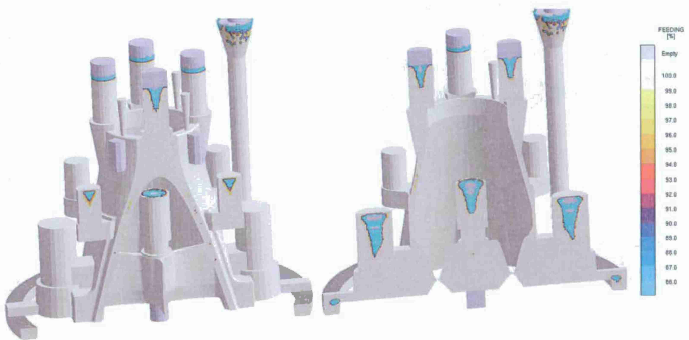
Figure 9 Additional slice views showing feeding shrinkage in risers and much smaller amounts in casting.
