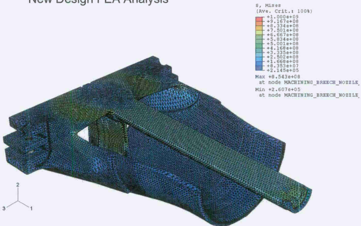
Figure 3 Von Mises stress distribution results on casting design.
