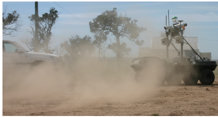
Fig. 6. Experiments with adverse environmental conditions including presence of airborne dust.
