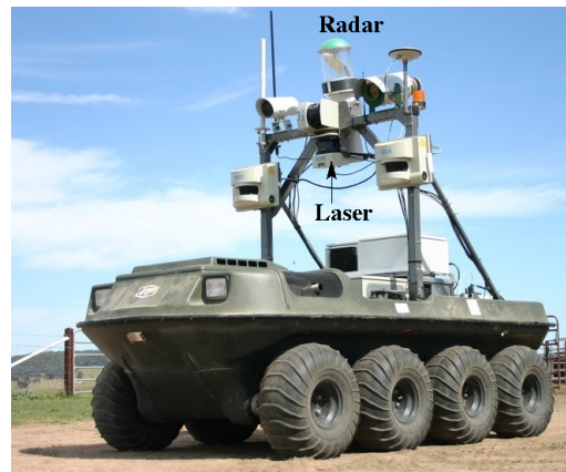
Fig. 4. The Argo UGV and its sensors.
