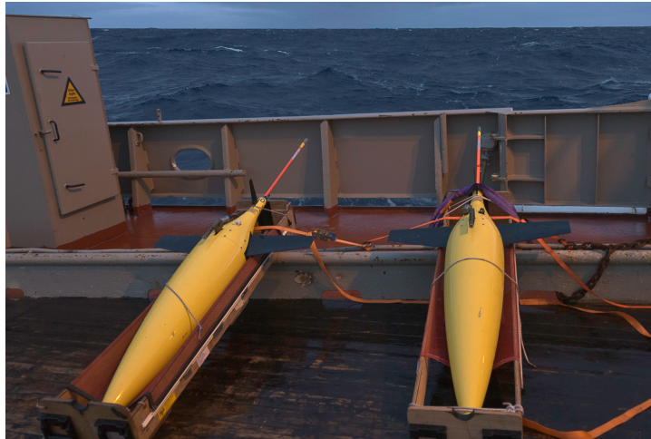
Figure 10. APL-UW ice-capable Seagliders. Gliders are small (50 kg, 1.5 m), long-endurance (multi-month), buoyancy-driven vehicles capable of navigating survey patterns while diving from the surface/ice–ocean interface to depths up to 1000 m. Iridium satellite modems provide two-way communications for command and data upload. Payload includes Seabird T & C, dissolved oxygen, downwelling irradiance, and temperature microstructure.
