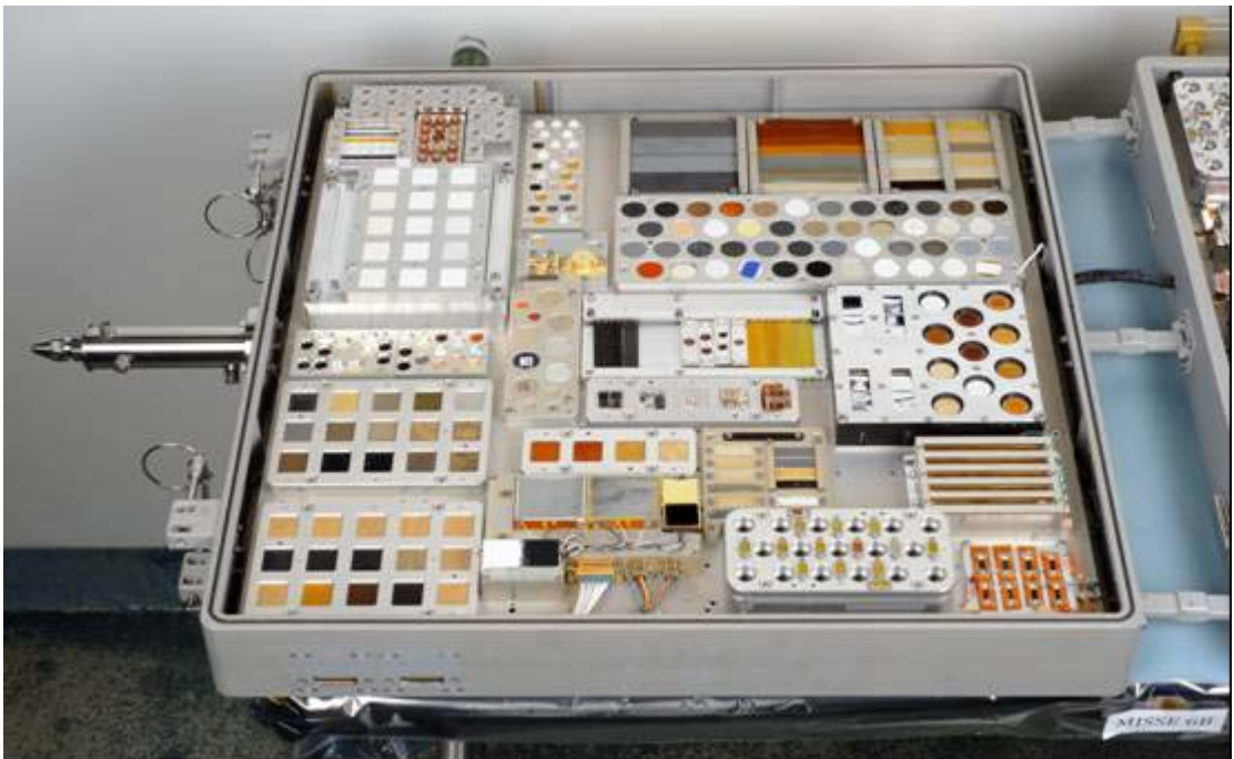
Figure 26. MISSE-6B, wake-facing side, post-flight (NASA Image).
