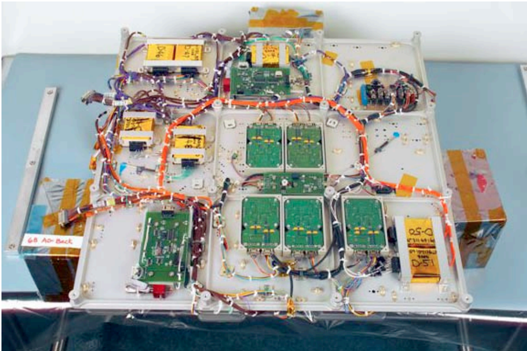
Figure 3. MISSE-6B AO side electronics attached to underside of tray holding experiments, preflight in the NASA LaRC clean room (NASA image).
