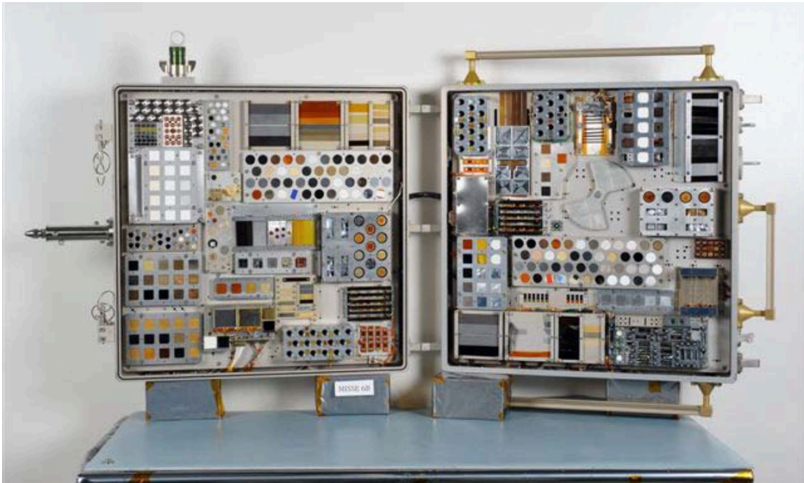
Figure 1. MISSE-6B preflight in the NASA LaRC clean room (NASA image).
