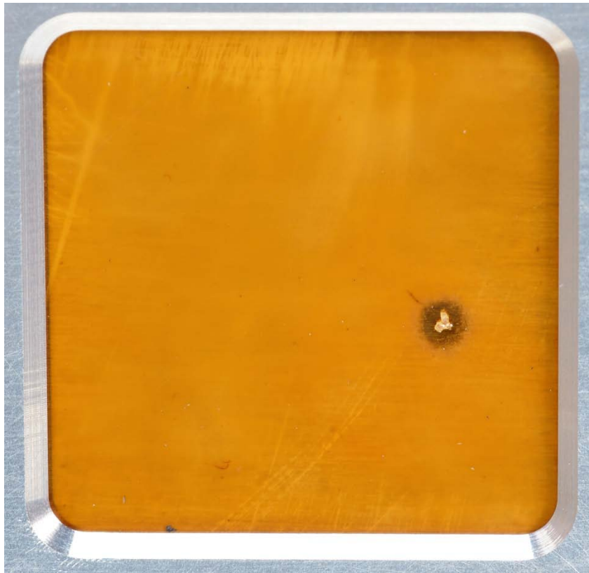
Figure 16. Impact in thin film specimen from MISSE-6 (NASA image).
