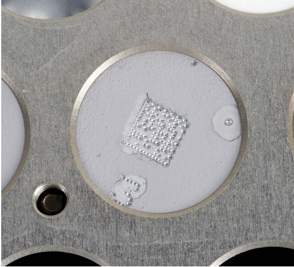
Figure 17. Impact on specimen from MISSE-6 (NASA image).
