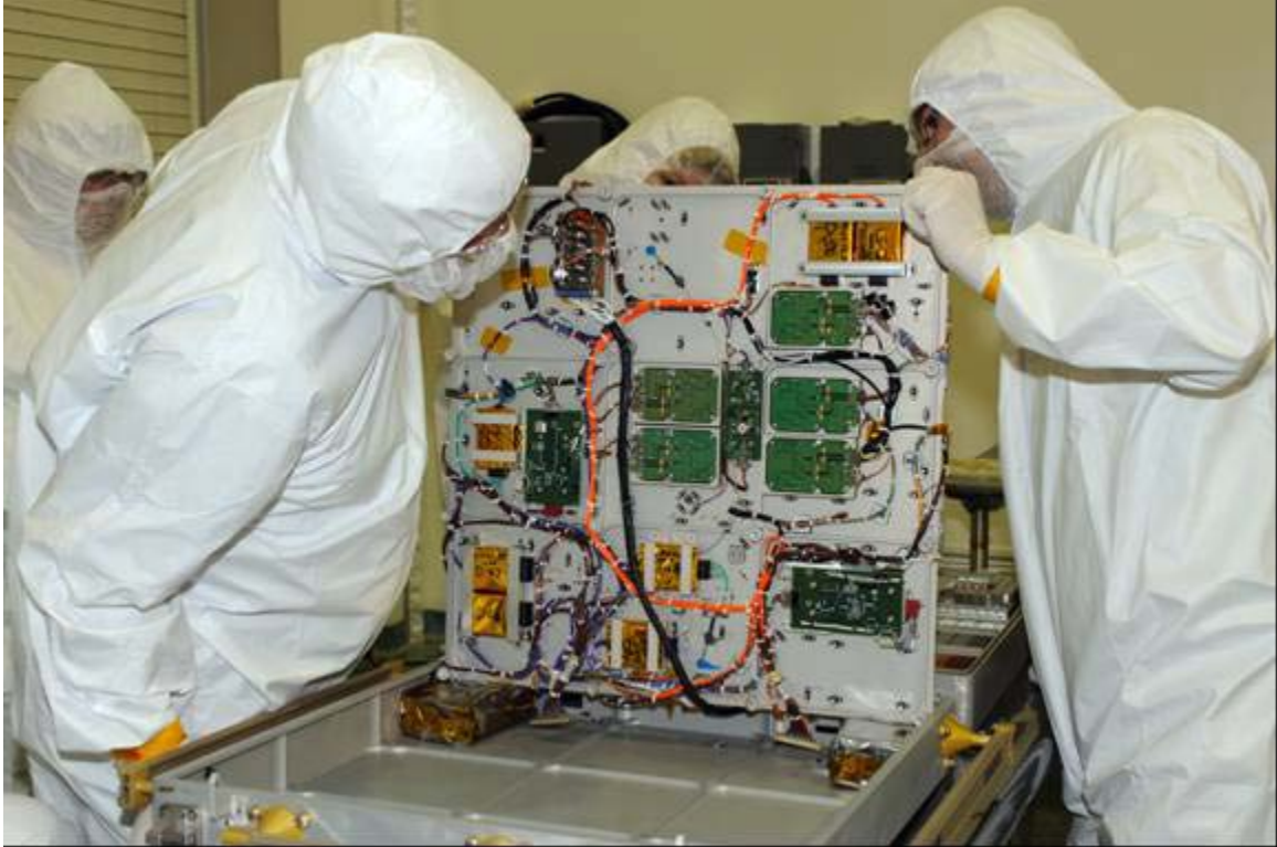
Figure 27. Inspection of MISSE-6B tray from the ram-facing side, post-flight (NASA Image).
