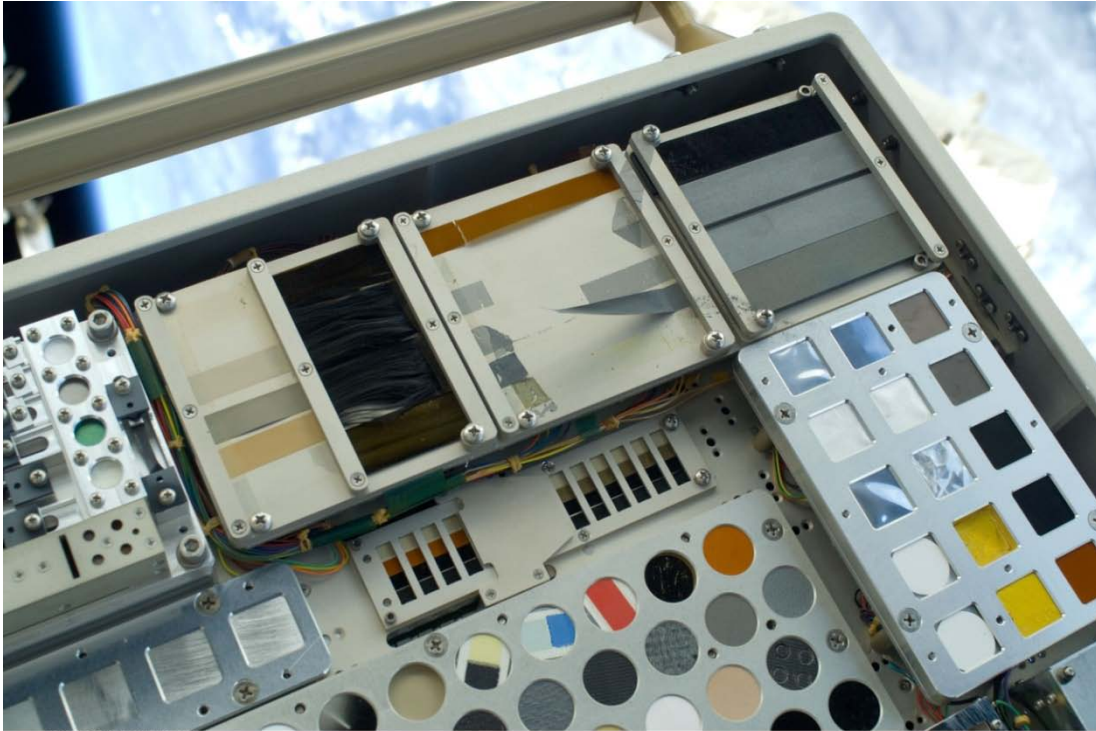
Figure 9. MISSE-6B AO/UV side on-orbit, showing damage to thin films (NASA image).
