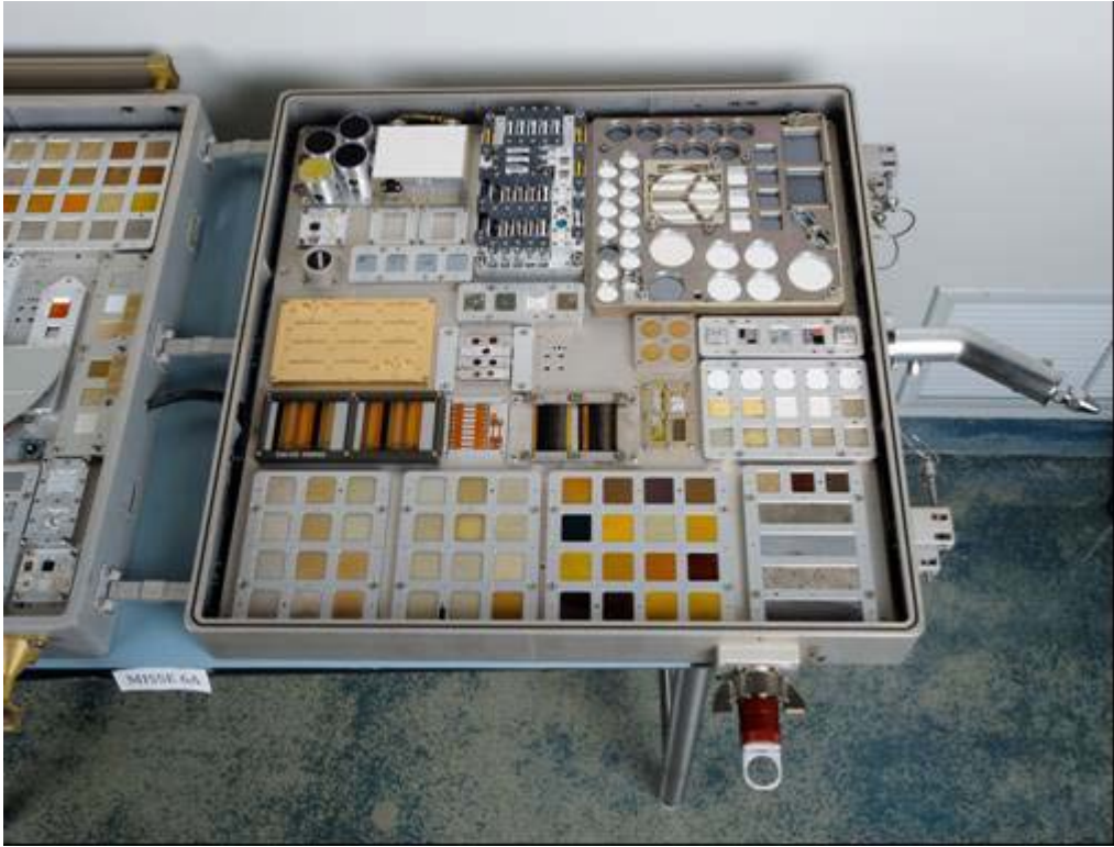
Figure 24. MISSE-6A, wake-facing side, post-flight (NASA Image).
