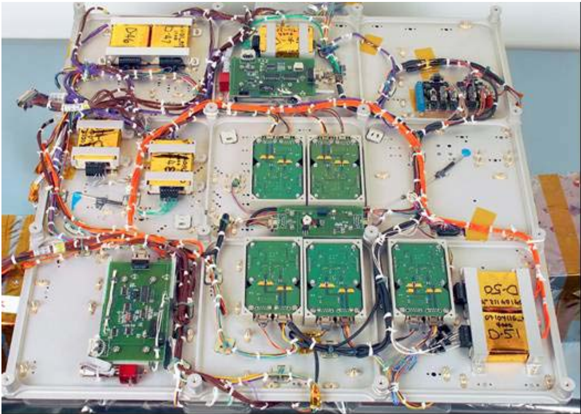
Figure 12. Location of thermistors on MISSE-6B AO/UV side tray.
