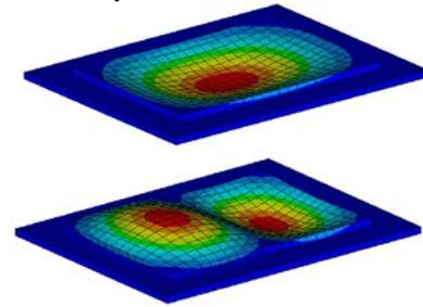
**Figure 6:** 1<sup>st</sup> and 2<sup>nd</sup> modes of a fixed-boundary cell
