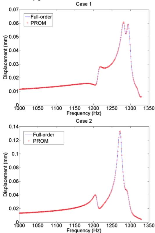
**Figure 8:** Forced response predictions for the 20<sup>th</sup> cell predicted by a full-order finite element model and a PROM for parameter variation Case 1 (top) and Case 2 (bottom)
