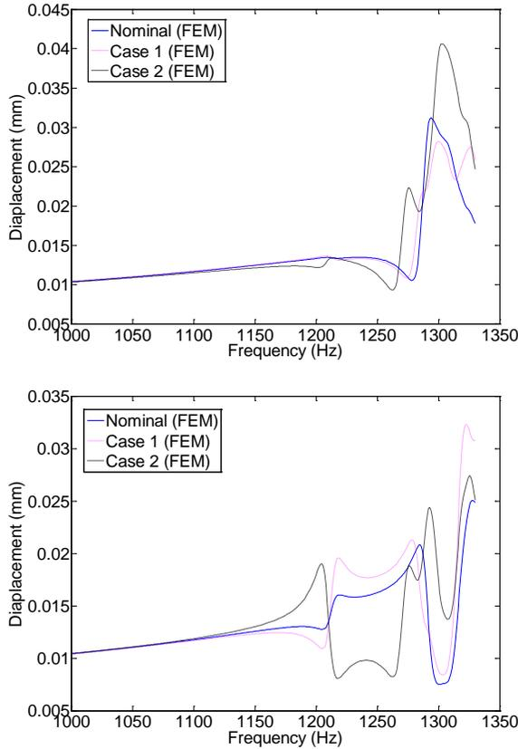
**Figure 5:** Forced response for the 10<sup>th</sup> cell (top) and 18<sup>th</sup> cell (bottom) of for the nominal case of no parameter variations versus two cases with parameter variations
