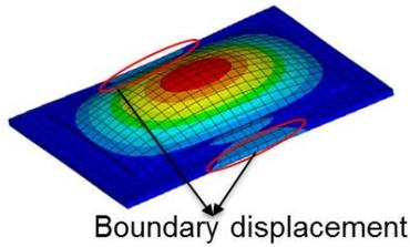
**Figure 7:** Boundary-displaced motion of a plate-like cell
