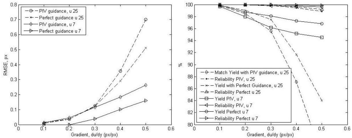
Figure 6 a) RMS Error, and b) percent yield and reliability vs. flow gradient for uniform shearing flow. Flows containing maximum displacements of  $\pm 7$  and  $\pm 25$  pixels are compared. The VB-PTV matching is guided both by PIV and exact analytic solutions.
