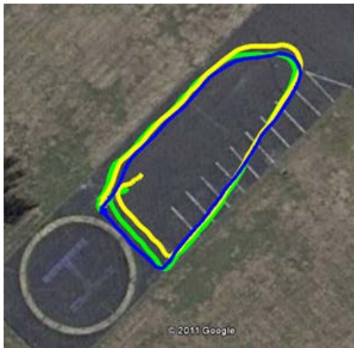
Figure 5: Loop closure test: Yellow – GPS, Green – GPR + RF; Blue – Visual Odometry.
