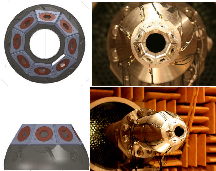
Figure 5: Drawings and in-situ photographs of nozzle with actuators
