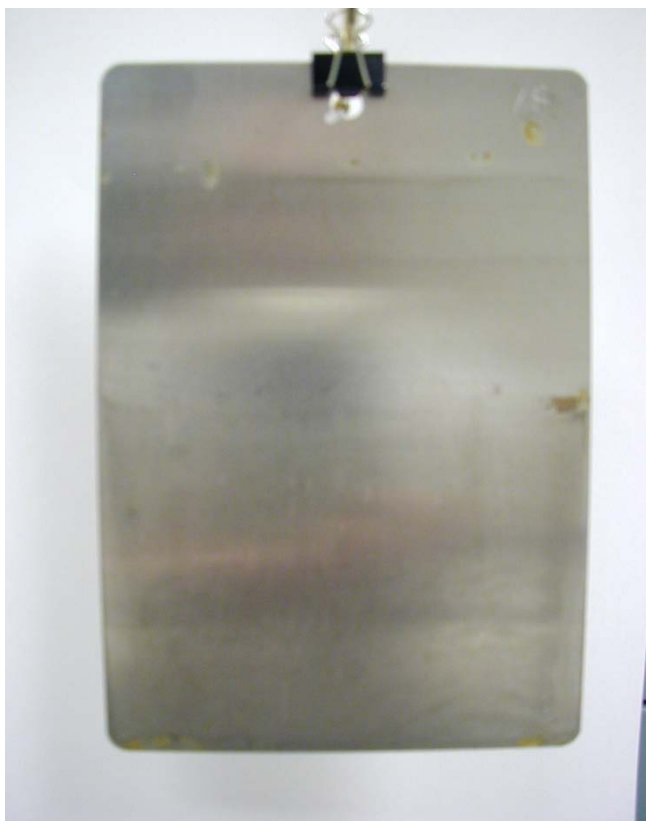
Bioclean coupon— ridge removed before solvent dip: Note flash rust.
