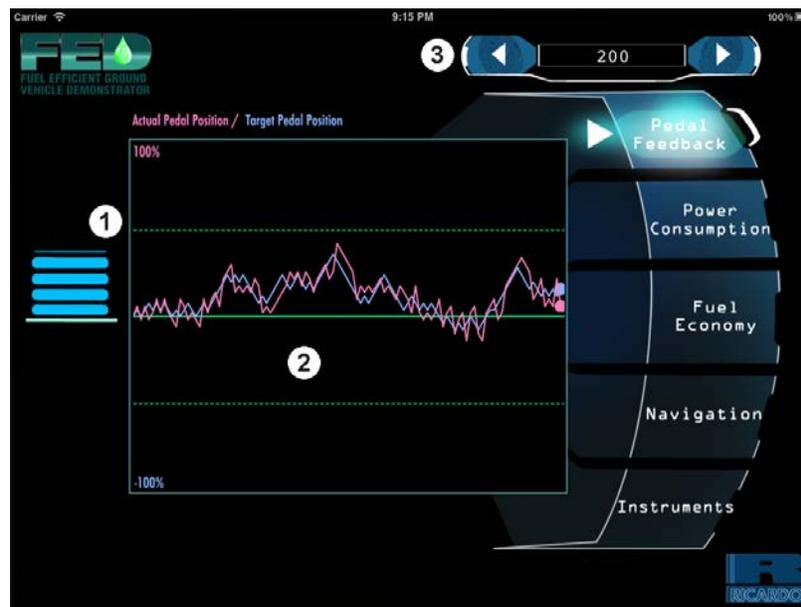
Figure 7: Pedal feedback screen showing pedal position indicator (1), time lapse graph of pedal displacement from target (2), and time scale (3)
