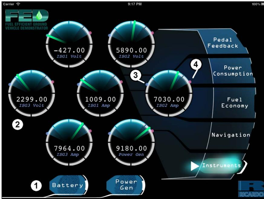
Figure 16: Instrument screen showing gauge type selection (1), individual gauges with numeric and text readout (2), minimum (3) and max (4) indicator
