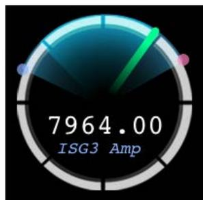
Figure 15: Close up of gauge, showing minimum value (blue dot), maximum value (red dot) and instantaneous value (green needle)
