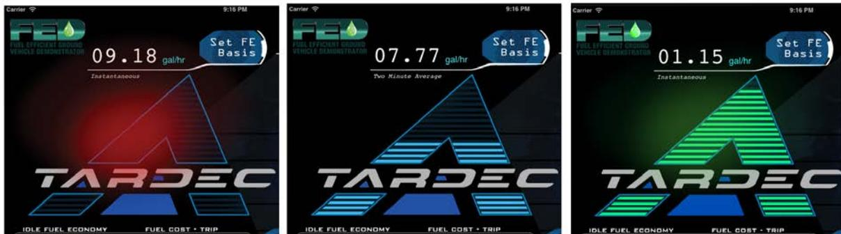
Figure 13: Fuel economy feedback indicators showing poor (left, red), nominal (middle, blue), and good (green, right) driving. Note the glow on red and green indicators.
