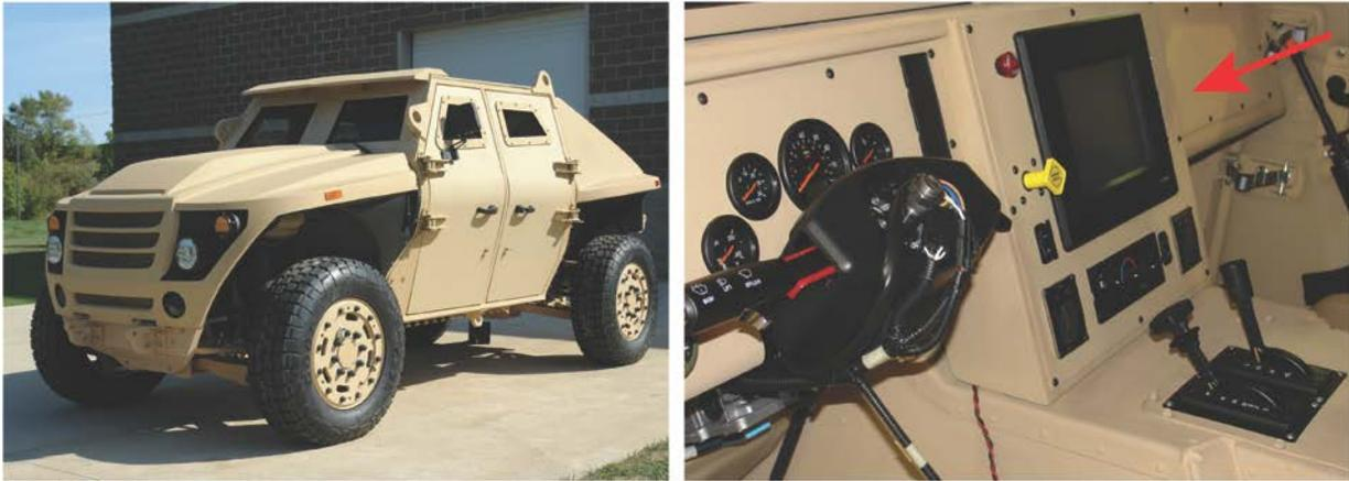
Figure 1: FED Alpha (Left) and Interior (Right) w/ In-Dash Vehicle Display
