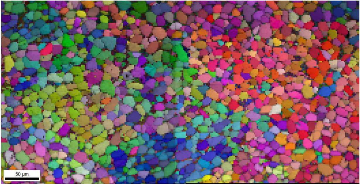
Figure 12. Crystal orientation map (see legend in Figure 6) of  $\alpha + \beta$  forged Ti-6Al-4V alloy combined with the correlation shown in Figure 11. The image quality overlay is used to highlight the seam between the tiles which is in approximately the center of the image.
