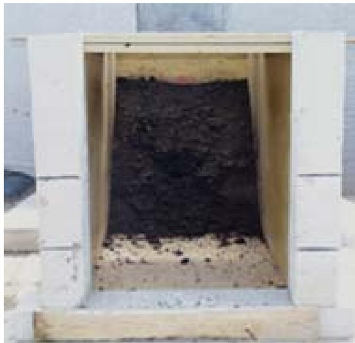
Figure 6. A live-fire lysimeter cell.
