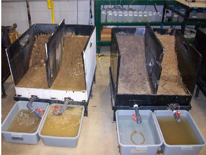
Figure 4. Slope stability boxes with unamended control cells on left and 0.2% biopolymer cells on right. The soil types in each pair are Silty Sand on left and Silt on right. Note the clarity of the leachate water from the biopolymer-amended soils on the right.
