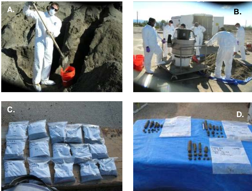
Figure 2. Sample collection, soil sieve separation, and sample preparation sequence from Catch Box areas 1 through 3.
