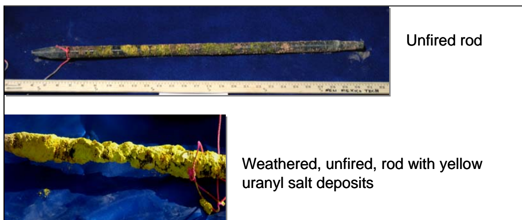
Figure 1. Comparison of weathered and unweathered depleted uranium rods illustrating the formation of uranyl oxides and salts. Unfired penetrator rods can range from 10 to 50 cm in length, depending on the type of munition.
