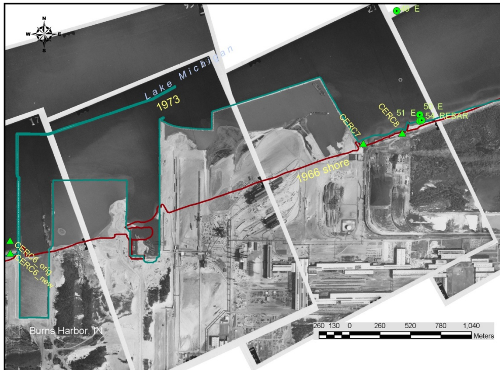
Figure 20. June 28, 1969. Burns Waterway Harbor under construction, with 1966 and 1973 shorelines to show extent of changes.
