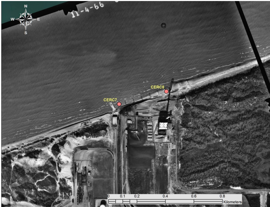
Figure 16. Shoreline at initial stage of Burnes Waterway Harbor construction, November 4, 1966. Bulkhead was under construction near CERC7.
