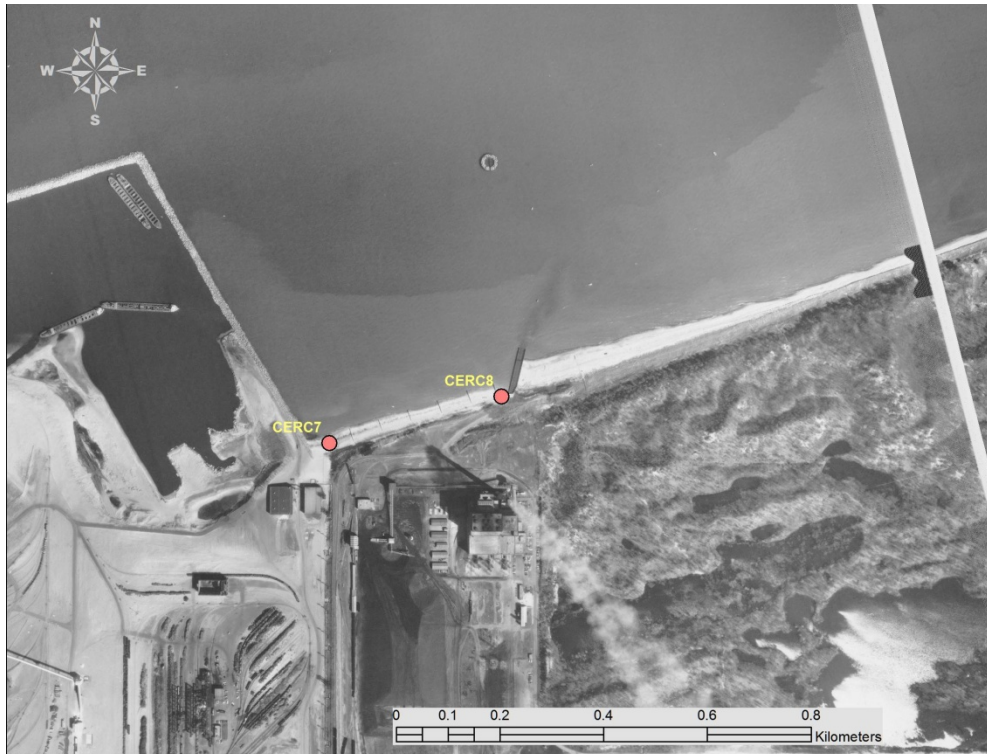
Figure 21. April 7, 1971. Sand had accumulated in and around the NIPSCO BGS groins compared to 1969.
