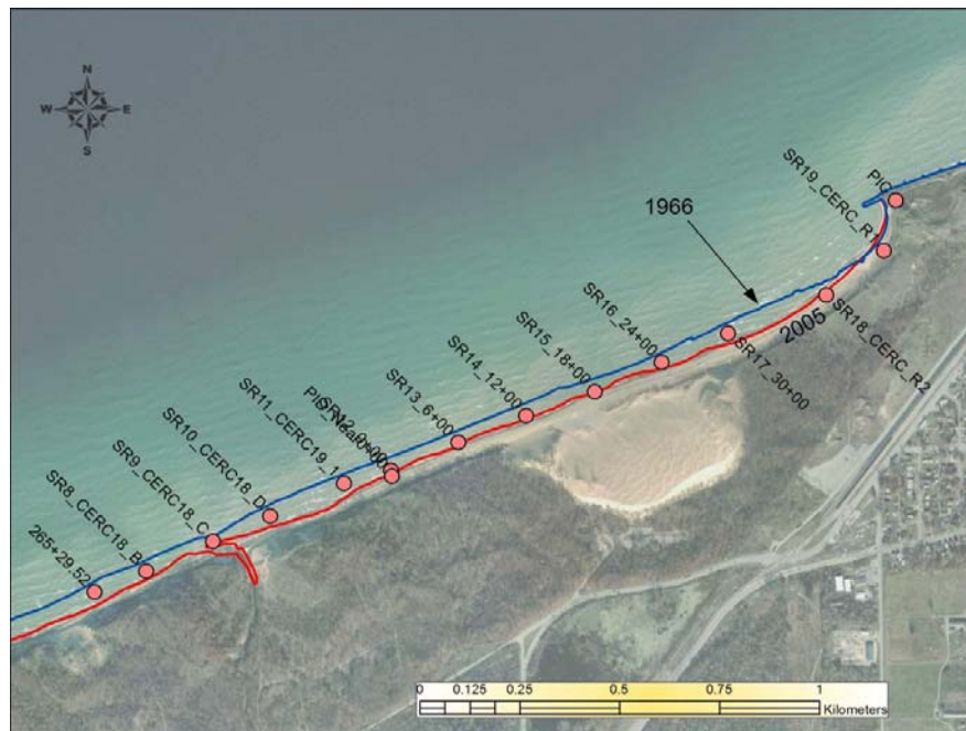
Figure 25. 1966 and 2005 +2 ft LWD IGLD1985 shorelines in the Mt. Baldy area, showing overall shore retreat. A shoreline (not available) from before the 50-year nourishment program was initiated in 1996, would have shown a much greater retreat. The 1996 pre-nourishment shore position can be approximated by the dark line (or shadow on the dune face) located between the trees still remaining at the top of the eroded dune face – and the lighter colored sand of the wide 2005 beach.
