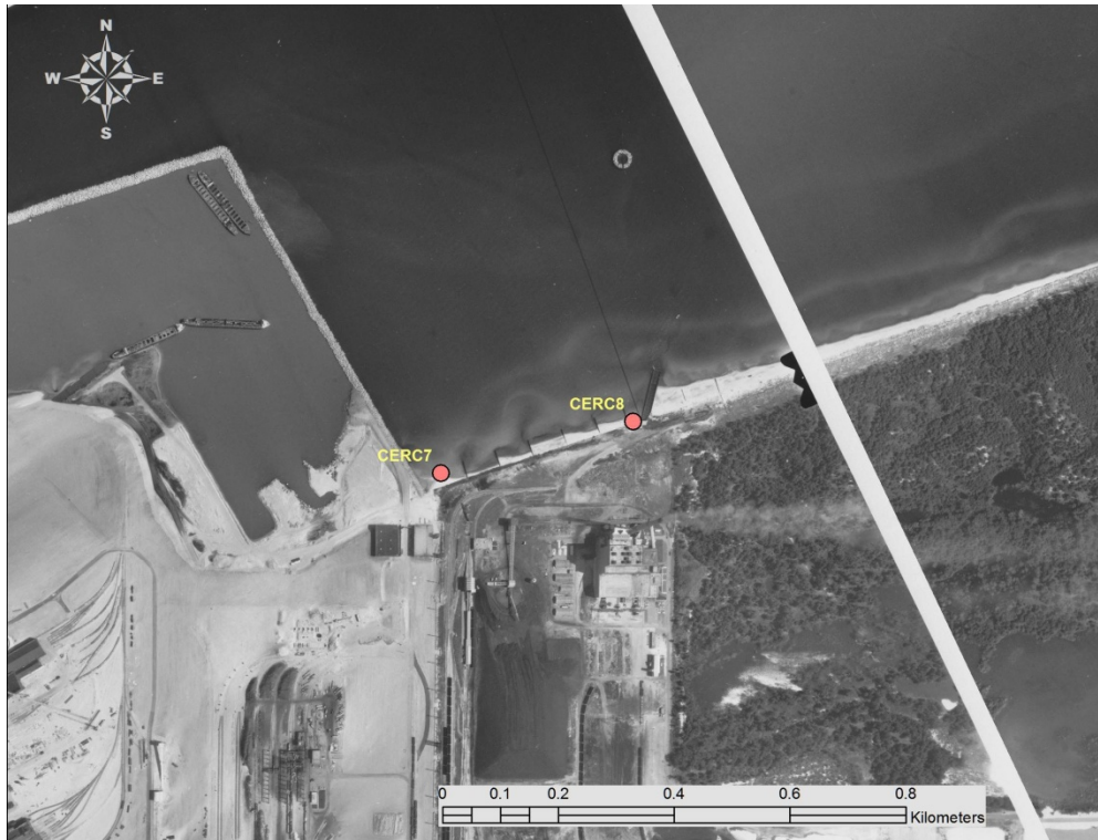
Figure 19. June 28, 1969. The Bethlehem Steel bulkhead was finished and former lake nearshore was being filled with sand. The shoreline shows some additional trapping east of the NIPSCO BGS outfall canal and minor loss between the cross-shore groins near CERC7. White line is border of photographic print.
