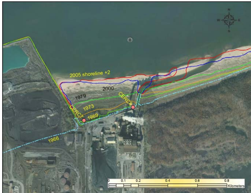
Figure 24. October 2011 (specific date not listed, from ESRI Maps and Data). The fillet extended to about half the length of the Arcelor-Mittal (formerly Bethlehem Steel) bulkhead, but the shoreline had not changed greatly since 2005. All shorelines represent +2 ft LWD IGLD1985.
