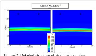
Figure 2. Detailed structure of stretched counterflowing air-hydrogen flame
